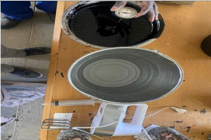
Checking the temperature of hot binder
