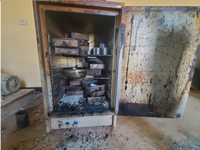
Heating of aggregate and asphalt binder
