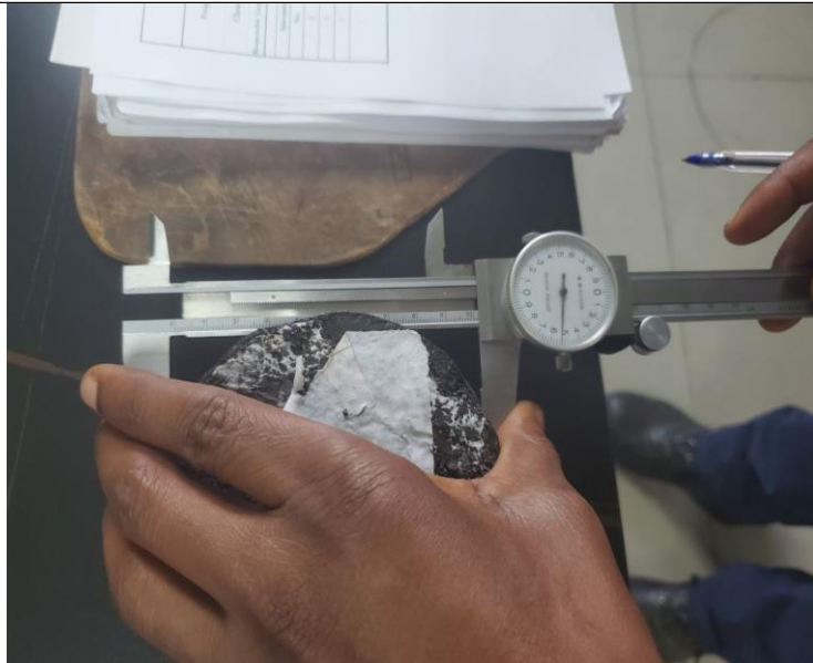
Measuring of thickness and diameter of the specimen
