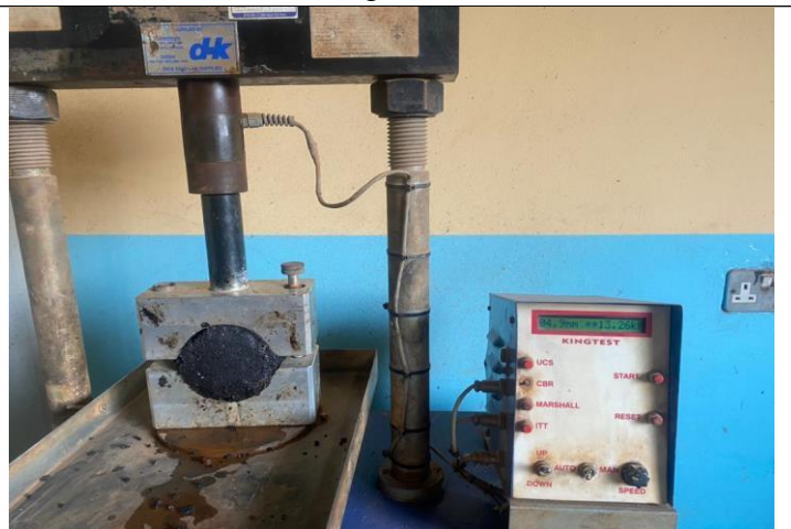
Testing for Marshall Stability and Flow
