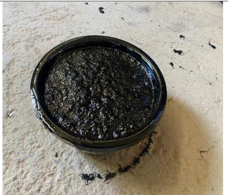
Foamed Asphalt Binder
