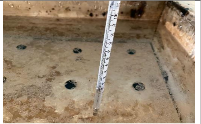
Checking of temperature @60 °C for soaking
