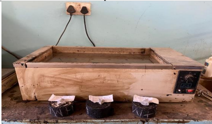
Hot water bath @ 60 °C
