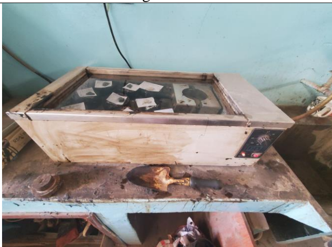
Soaking of specimens at 60°C
