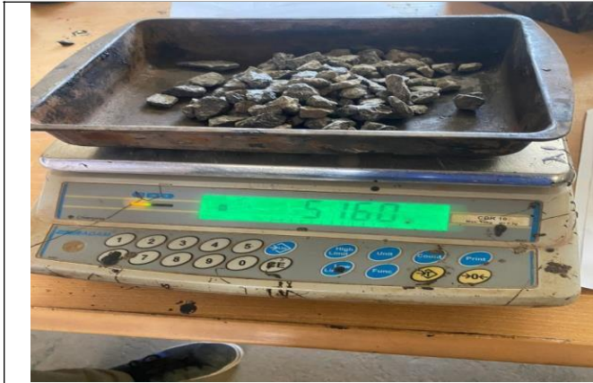
Weighing of aggregates as per blending proportions
