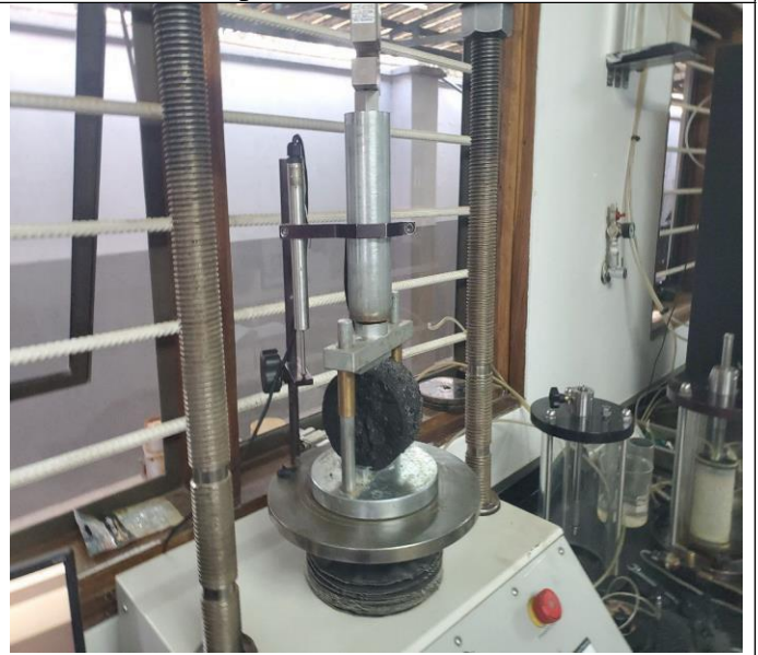
Testing for indirect tensile strength
