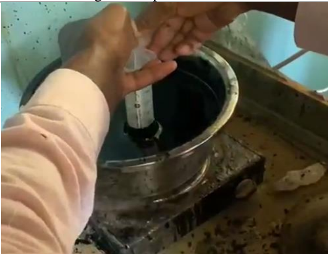
Injecting cold water to the hot binder
