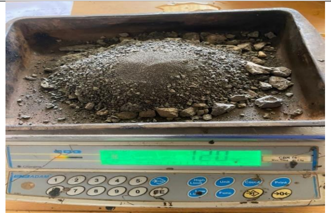
Weighing of aggregates as per blending proportions
