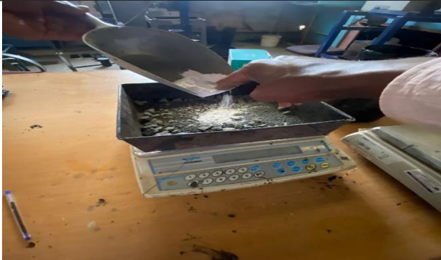
Adding of dry lime in a pre-mix process
