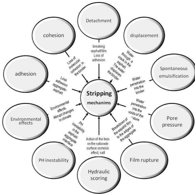
FIGURE 2. MECHANISMS OF STRIPPING
