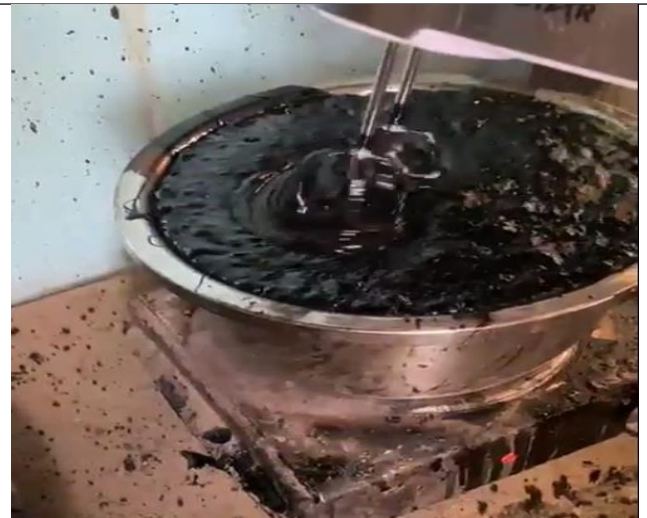
Mixing of the water and hot binder to create foam
