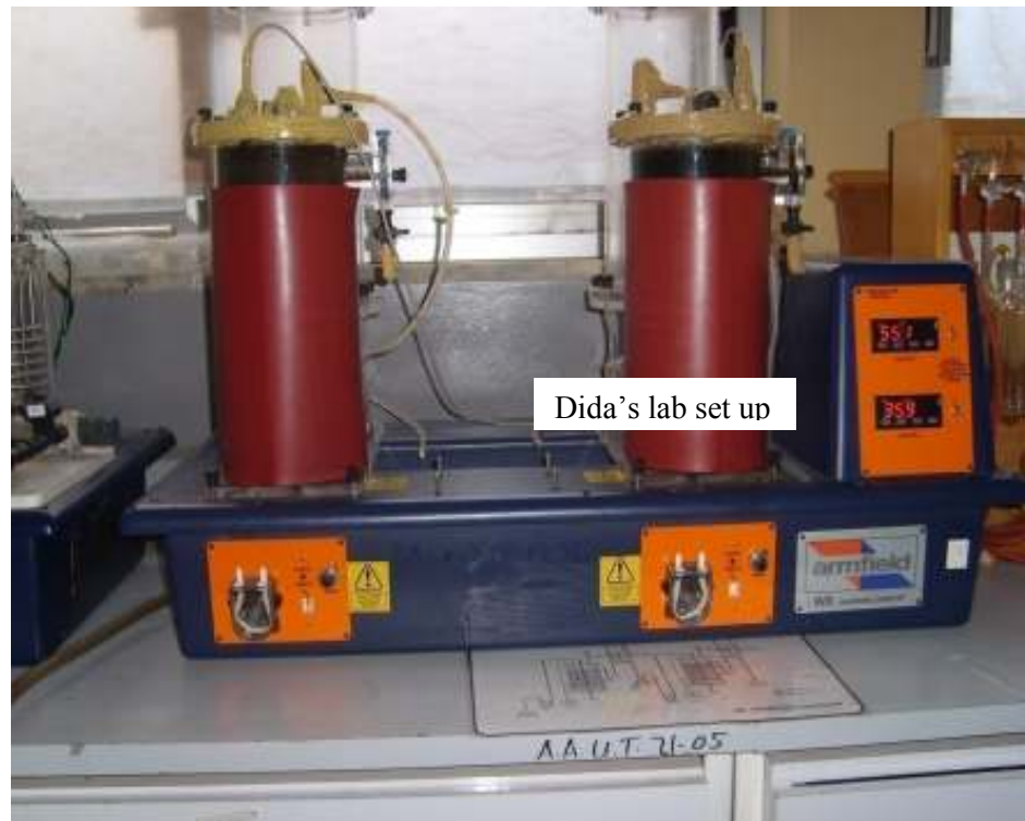
Fig. 3.5. Anaerobic digester used in the laboratory
