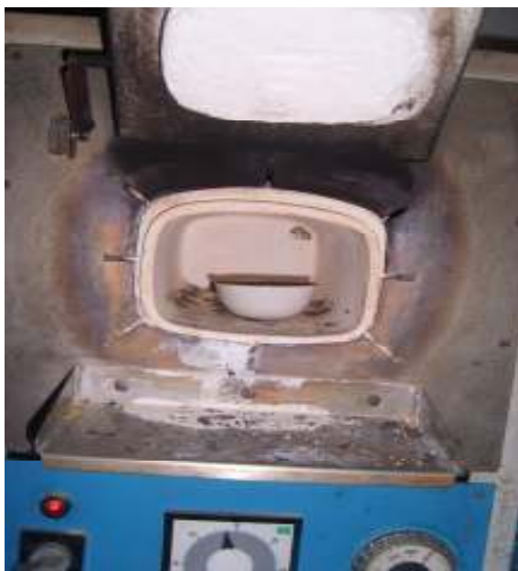
Fig.3.4. VS analysis in Muffle furnace
