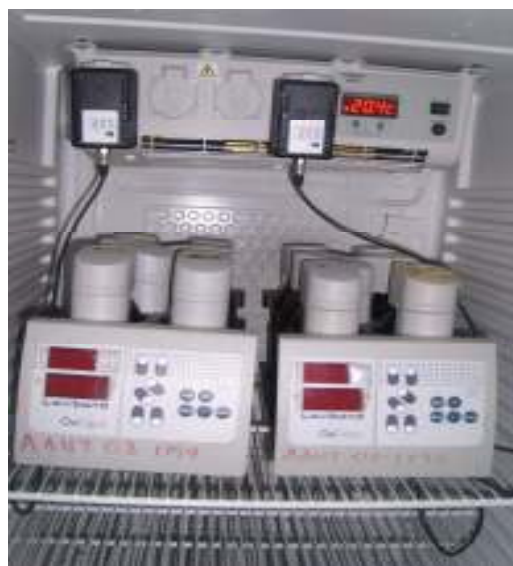
Fig. 3.2. BOD 5 under analysis
