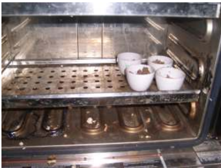
Fig.3.3. Sample in the oven for TS analysis
