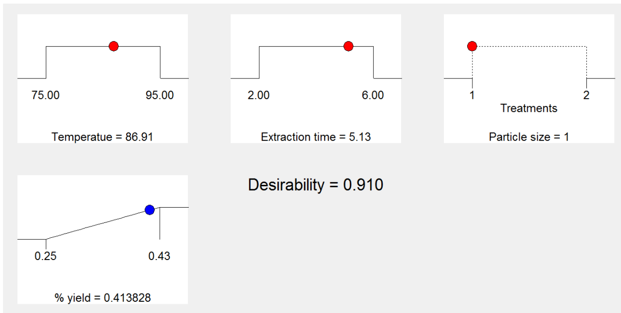
Figure 4.12: The highest yield offering treatments at particle size <1 mm in ramp form
