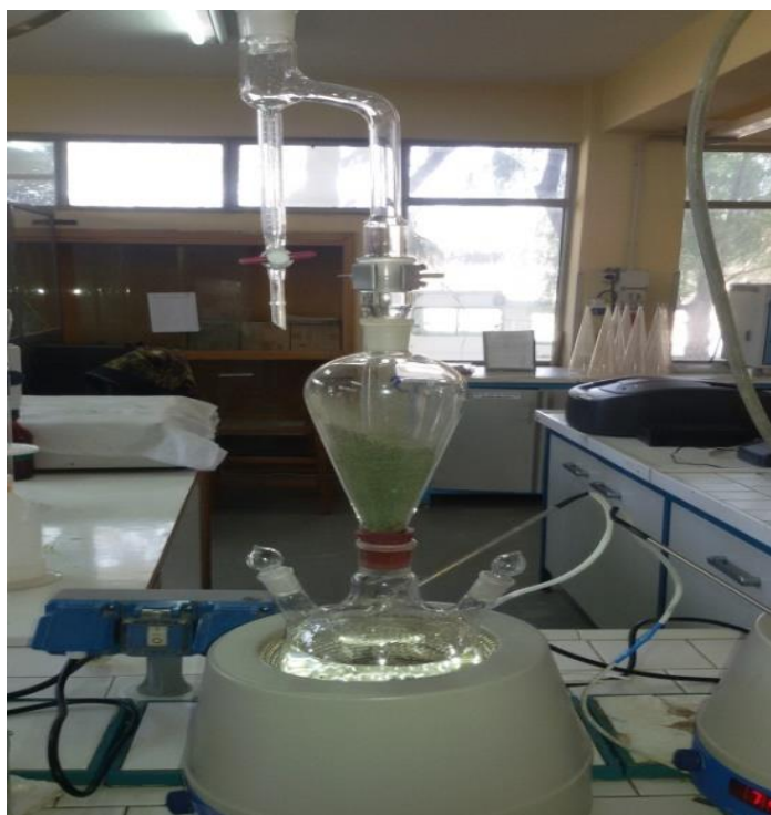
Figure 3.1: Experimental set-up for steam distillation of essential oil
