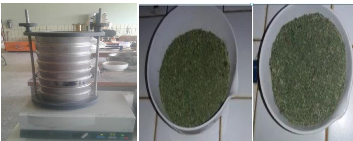
Figure G.2: Sieves analysis and samples of different particle size for extraction
