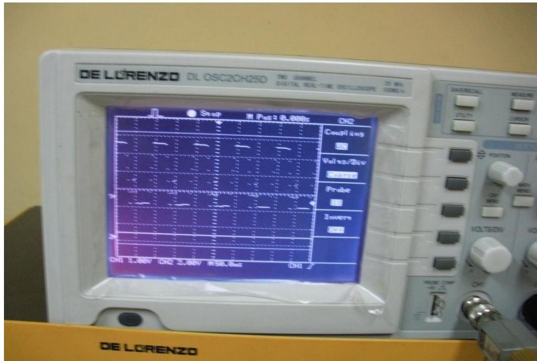
Figure 4.16: sample SVPWM output from the DSP
