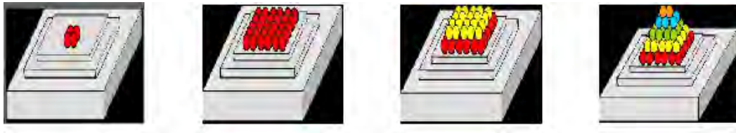
Figure 1.2: Si nanostructure grow continuously from smaller vertically layer- by-layer to large grid [5].
