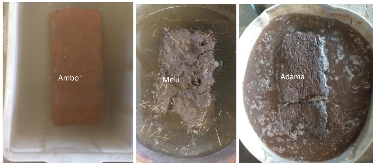
Figure 4.16: Mud block after soaked in water for 24hrs
