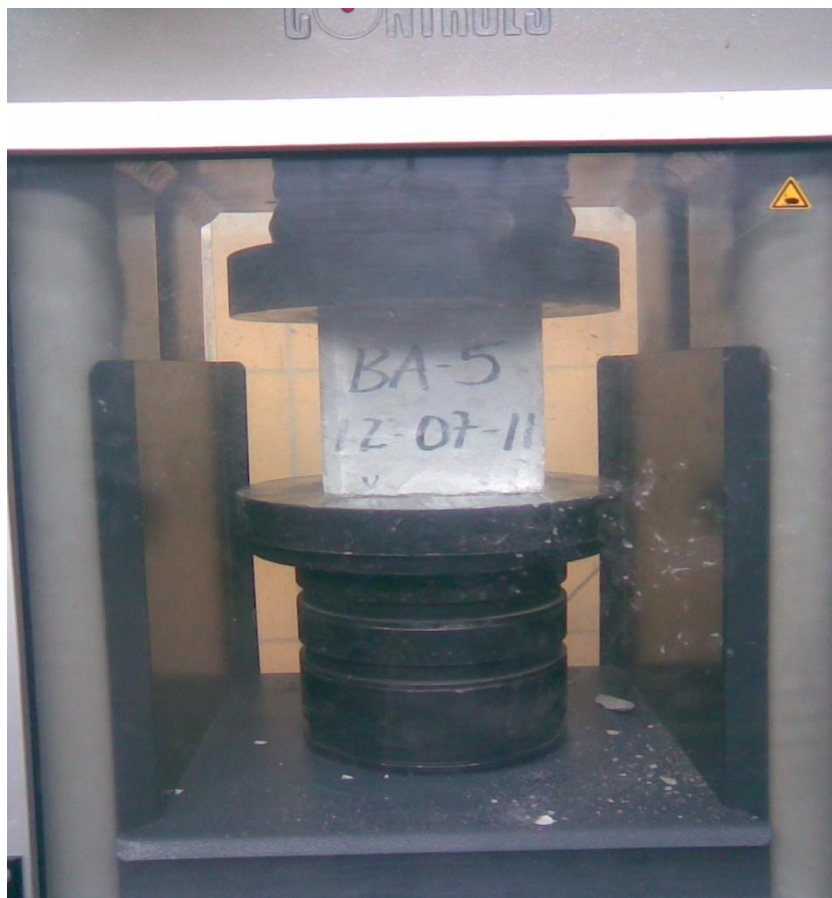
Photo 16. Concrete compressive strength test
