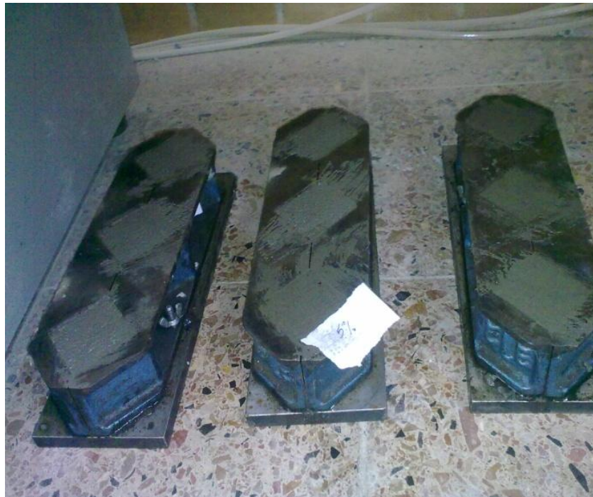
Photo 10. Mortar specimens after casting
