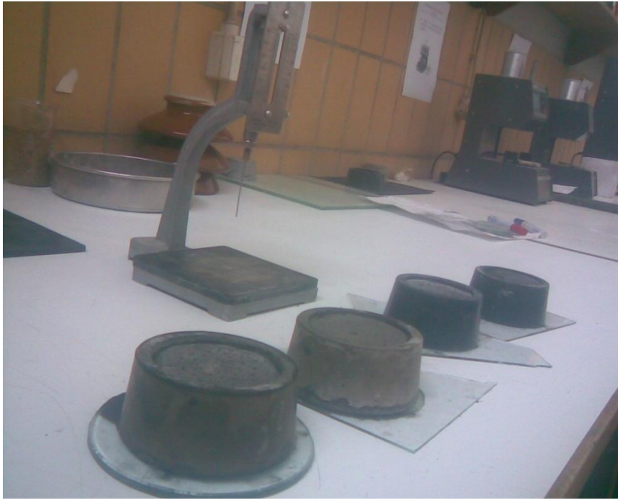
Photo 3. Setting time test under progress
