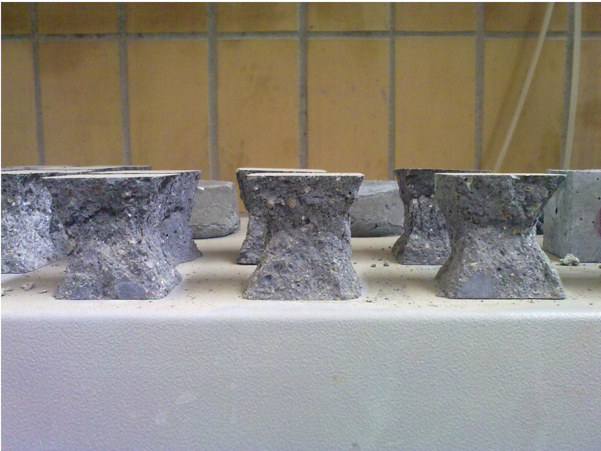
Photo 4. Mortar specimens after compressive strength test
