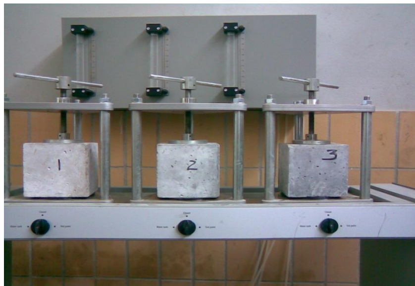
Fig. 5.9 Specimens ready for water permeability test
