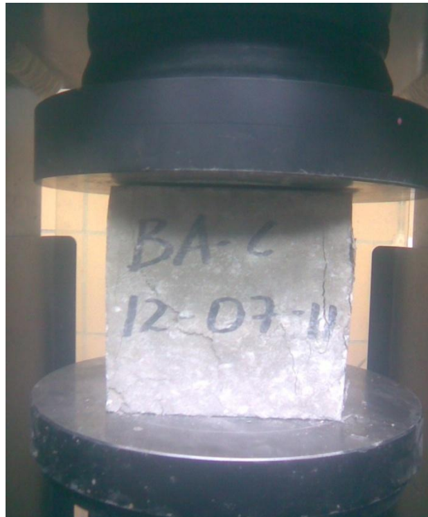
Fig.5.6 Compressive strength of concrete being tested
