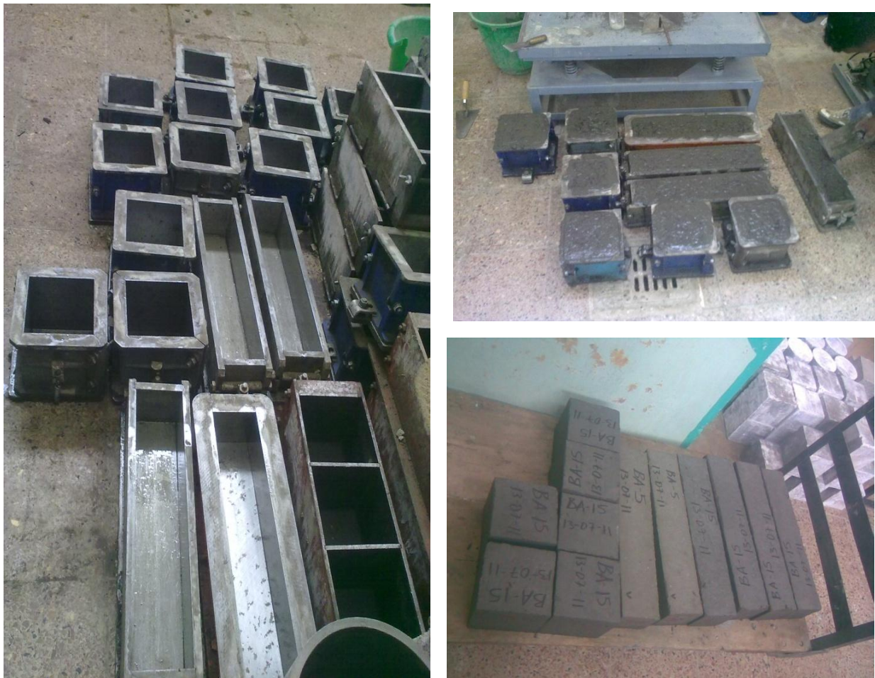
Photo 12. Oiled concrete molds (left), concrete specimens being trowled (top right) and concrete specimens ready to be cured (bottom right)
