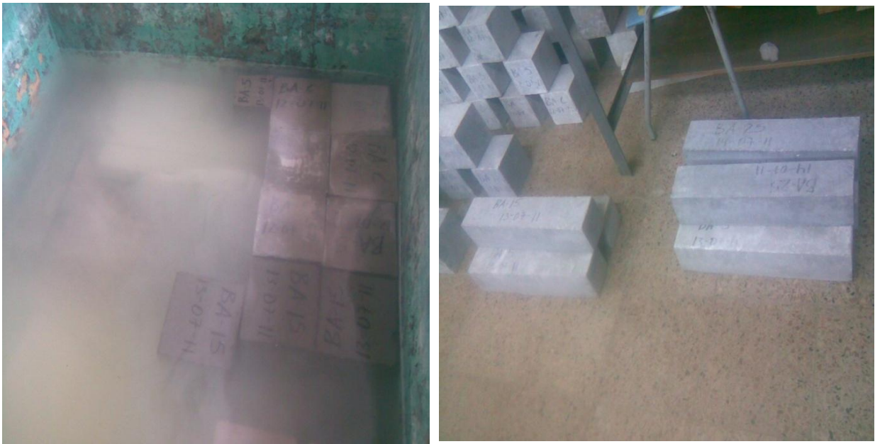
Photo 13. Concrete specimens in curing pond (left) and after curing (right)
