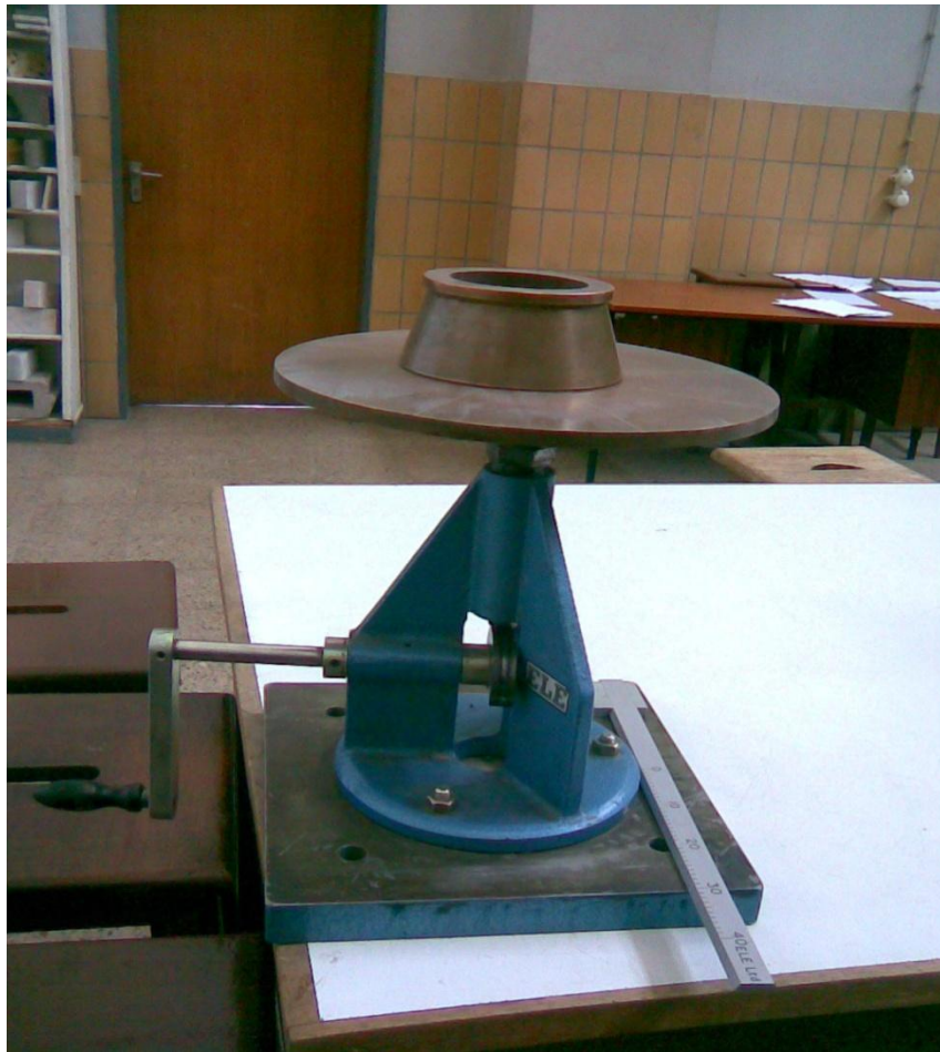
Photo 9. Flow table apparatus for mortar
