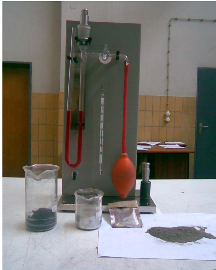
Photo 5. Blain air permeability apparatus and materials to be tested
