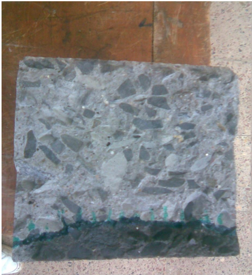
Fig. 5.10 Typical concrete sample just after splitting at the end of the water penetration test
