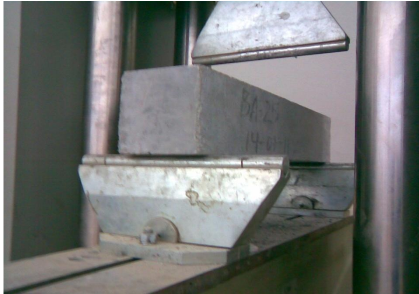
Fig. 5.8 Specimen to be tested for flexure
