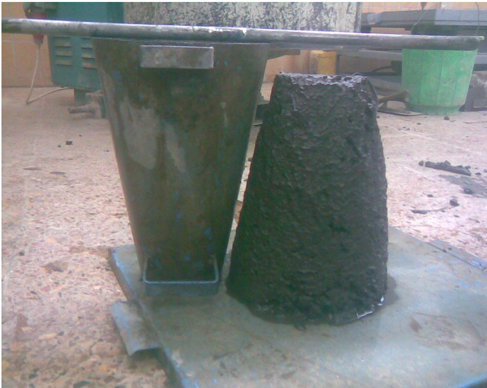
Fig. 5.4 Slump test of concrete
