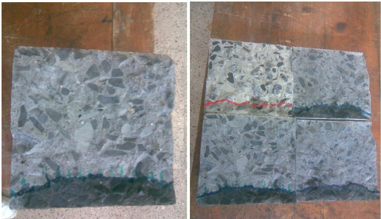
Photo 18. Water penetrated concretes
