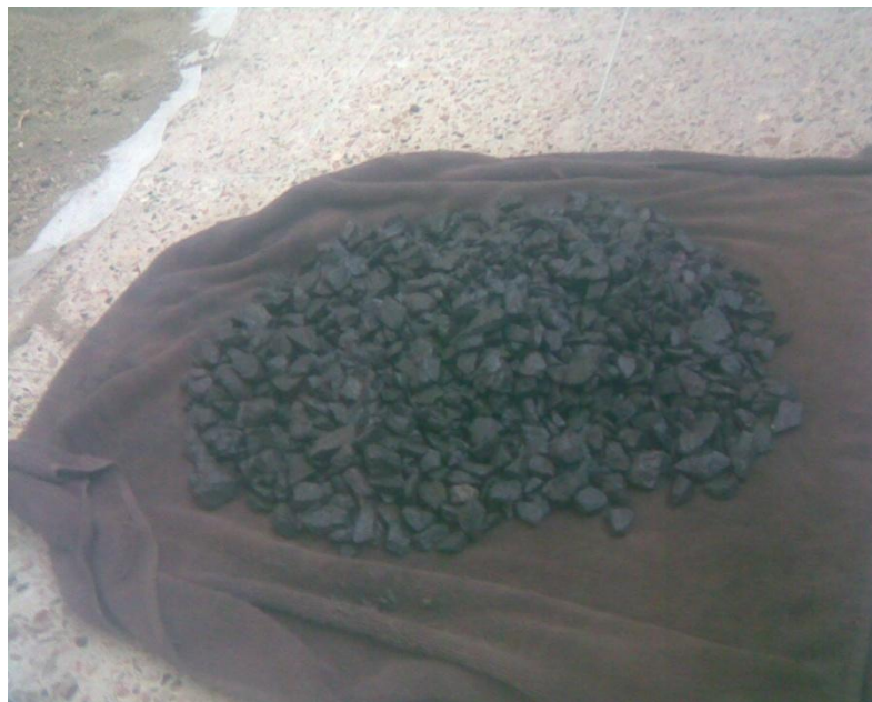
Photo 6. Coarse aggregate under specific gravity test
