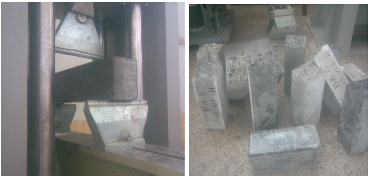
Photo 14. Concrete specimen to be tested for flexure (left) and concrete flexural specimen after failure (right)
