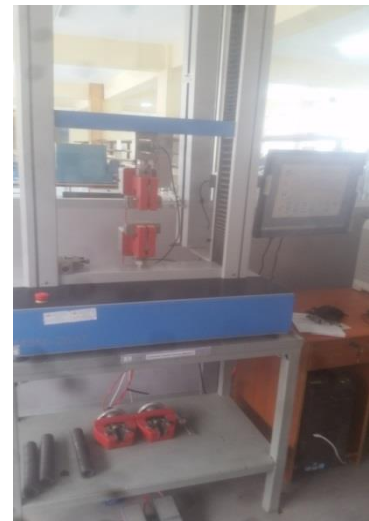
Universal testing machine to test the tensile and tear strength
