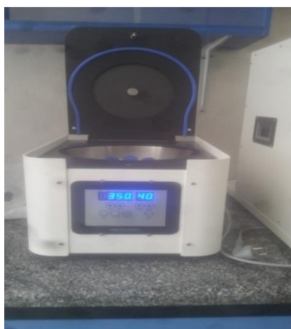
Centrifuge to remove gum and phosphatides
