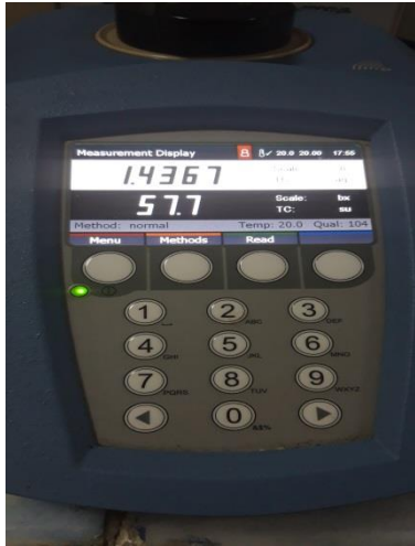
Refractometer measures Refractive index
