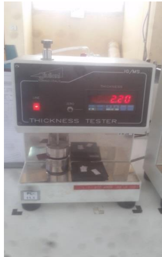
Thickness tester measures Thickness of crust sample
