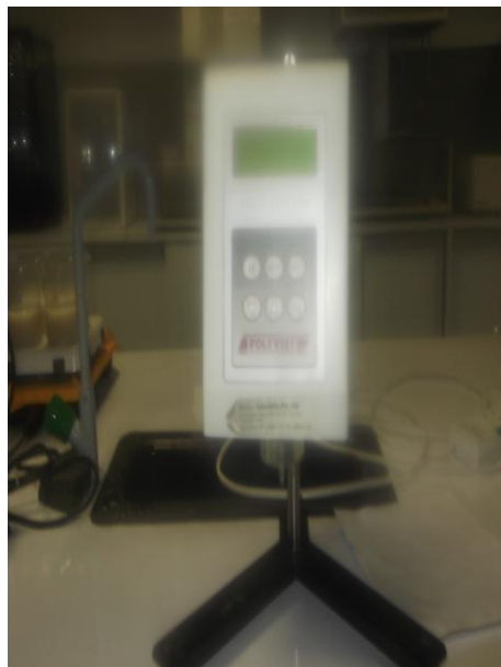
Fig 1. Polyvisc (model VS 003, type viscometer) was used to measure the viscosity of samples.
