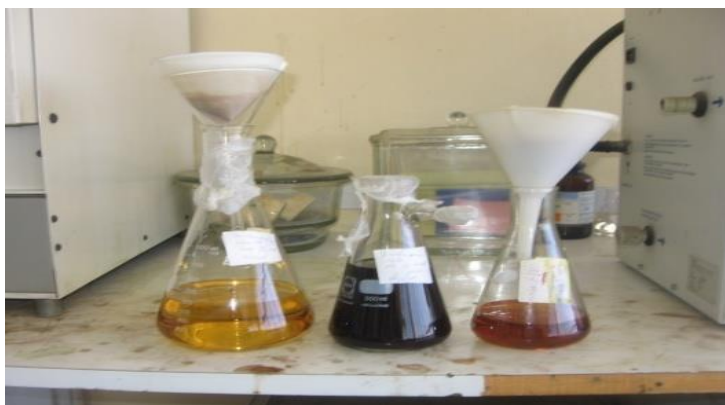
C: Samples filtered in Erlenmeyer flasks
