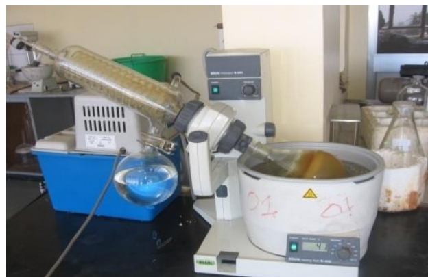
D: Buchi rota vapor (on condensation process)
