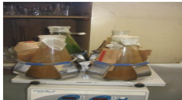
B: Rotary shaker adjusted at 140rpm
