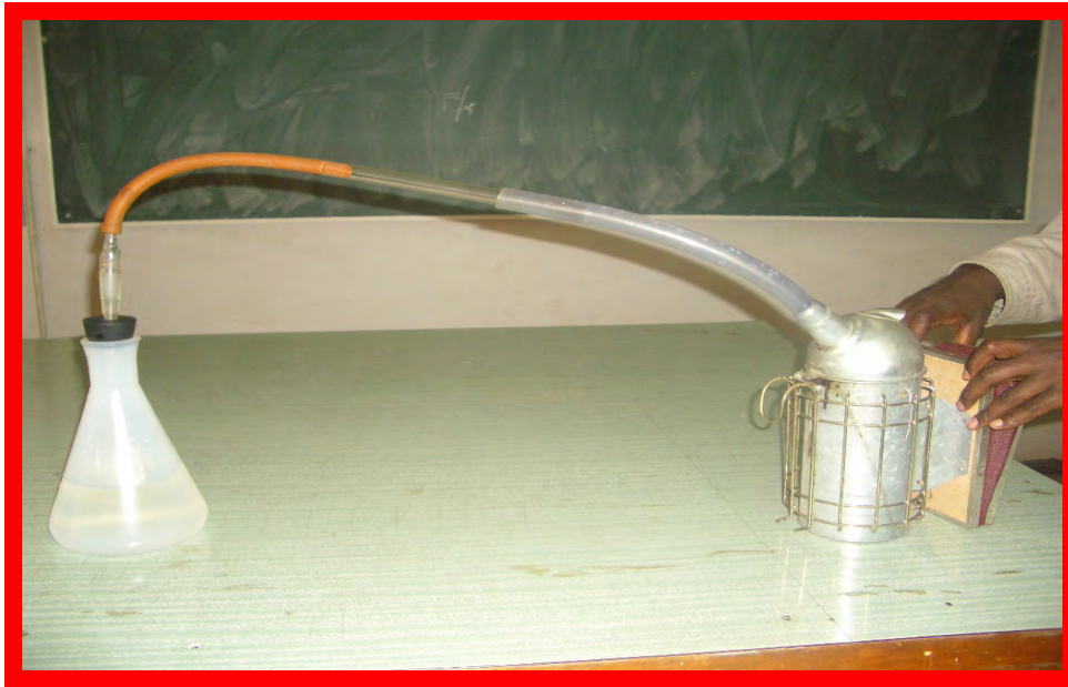
Figure 2. Arrangement of the apparatus used for smoke extraction.
