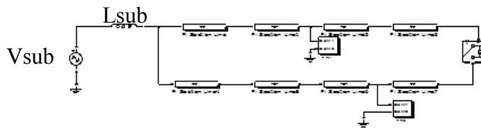
Figure 3.6: MATLAB/SIMPOWER Model of the traction system to be studied [author]
