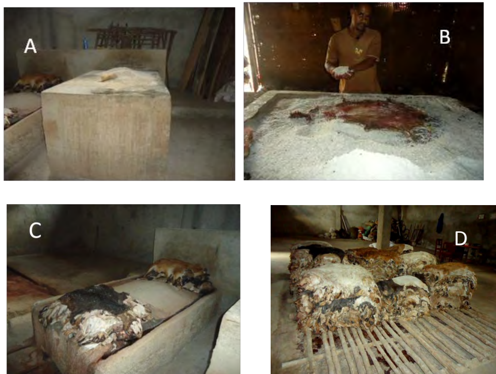
Figure 3: steps in curing of hides and skins
