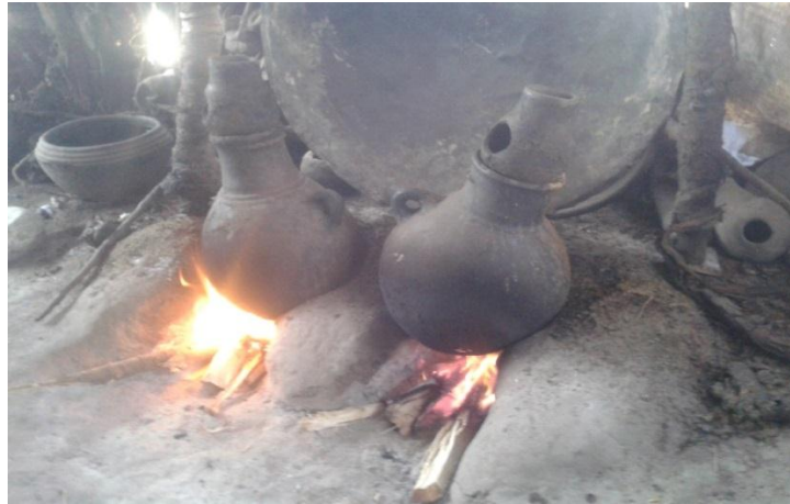
Figure 15 Photograph of difedif undergoing pre-heating process before sealed
