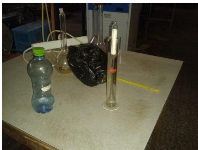
Figure 21 Specific gravity measurement of areke using hydrometer
