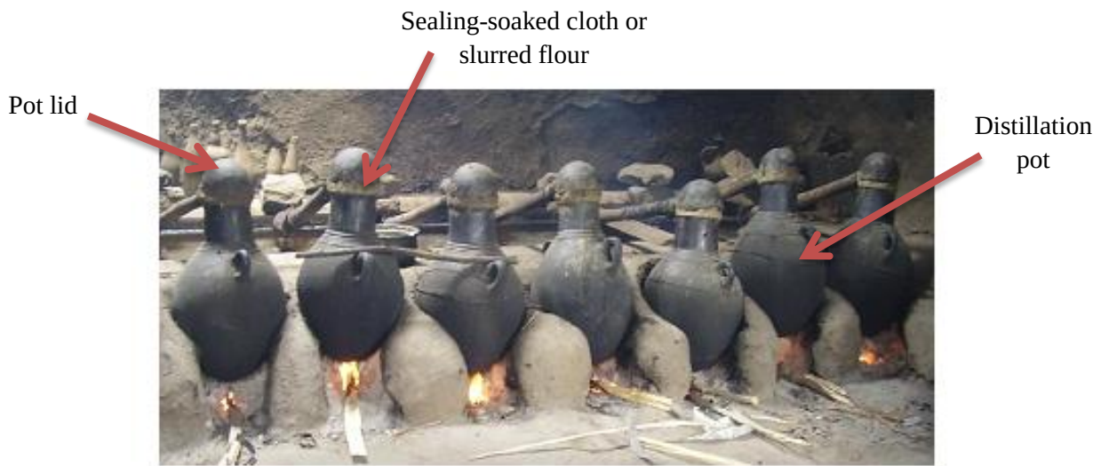
Figure 12 Multiple traditional areke distillation stove (rounded shape to hold the shape of pot) [9]
