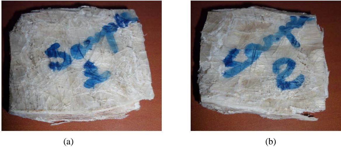
Figure 5.7: Compressive failure (a) specimen (NFC-1), (b) specimen (NFC-2)
