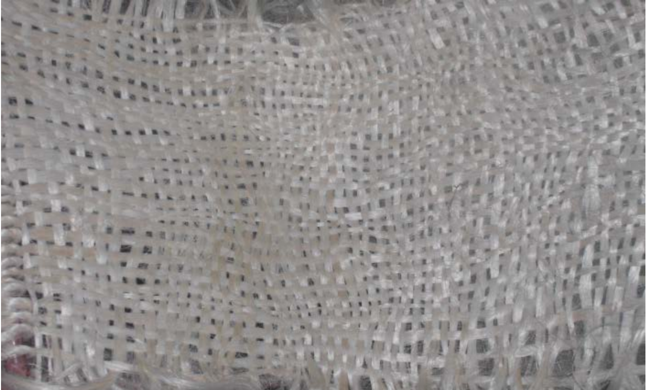
Figure 3.4: Special woven mat from bundles of fiber
