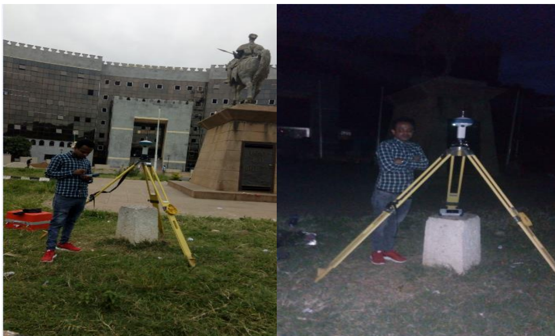
Figure 3.3. Static GPS field observation on GCP established by E.G.I.A.
