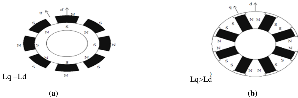
Figure 2:3 Rotor configurations: a) Surface Mounted PM (SPM); b) Interior PM (IPM) [1]
