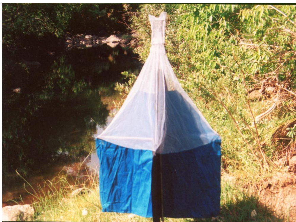
Image 2: Mono-conical trap fixed in the site of study to capture vector fly (tsetse and biting flies) during the study period
