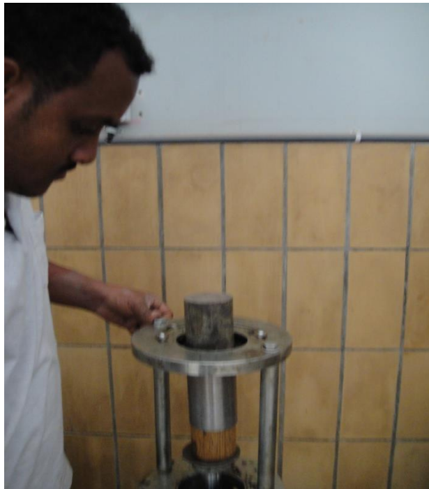
Figure B- 11 Extruding undisturbed soil sample from the sampling tube.
