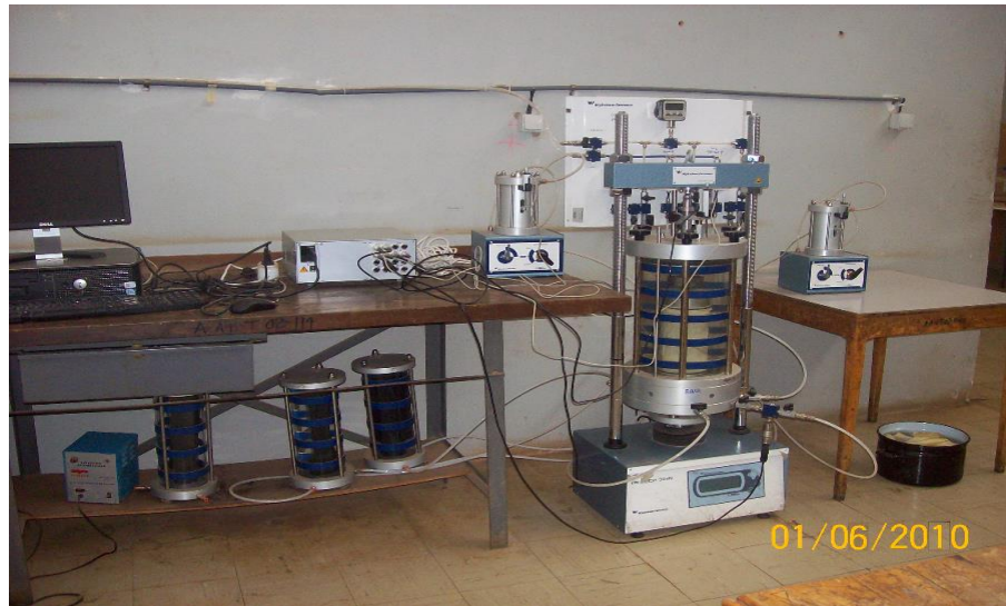
Figure 3.2 Modified triaxial machine
