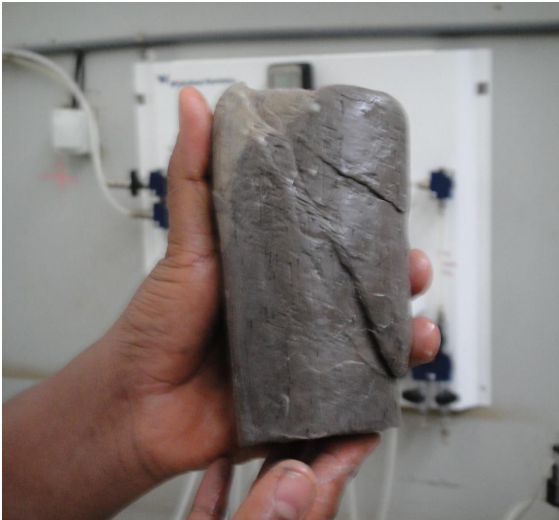
Figure B- 13 Soil sample after shearing
