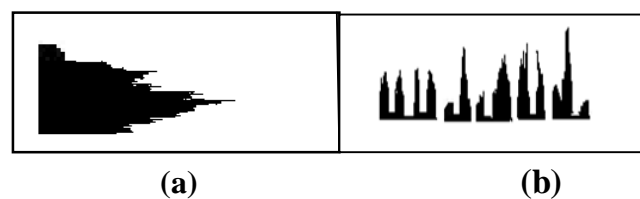
Figure4.2 Representation of the word mNGST in Horizontal (a) and Vertical (b) projections
