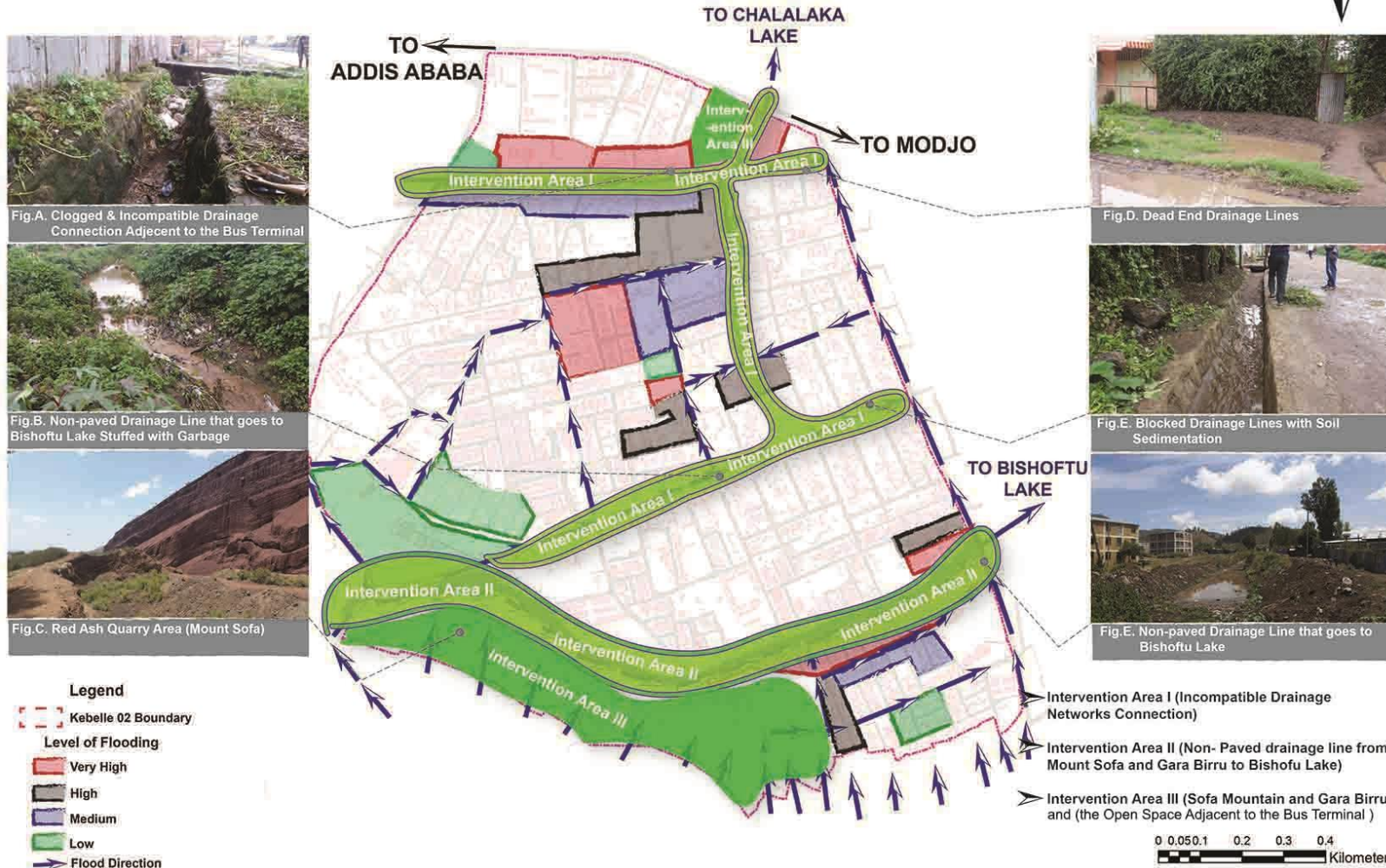
Figure 63 Possible Flood Prevention Intervention areas
