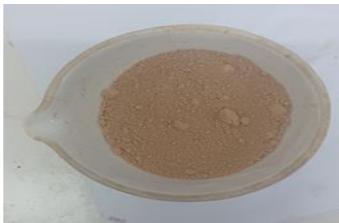
Figure 7 powdered textile sludge after calcination at 600 °C for 2 hours
