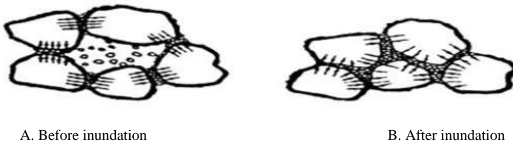
Figure 2-1 Structure of collapsible soils (Houston, et al.,1988)
