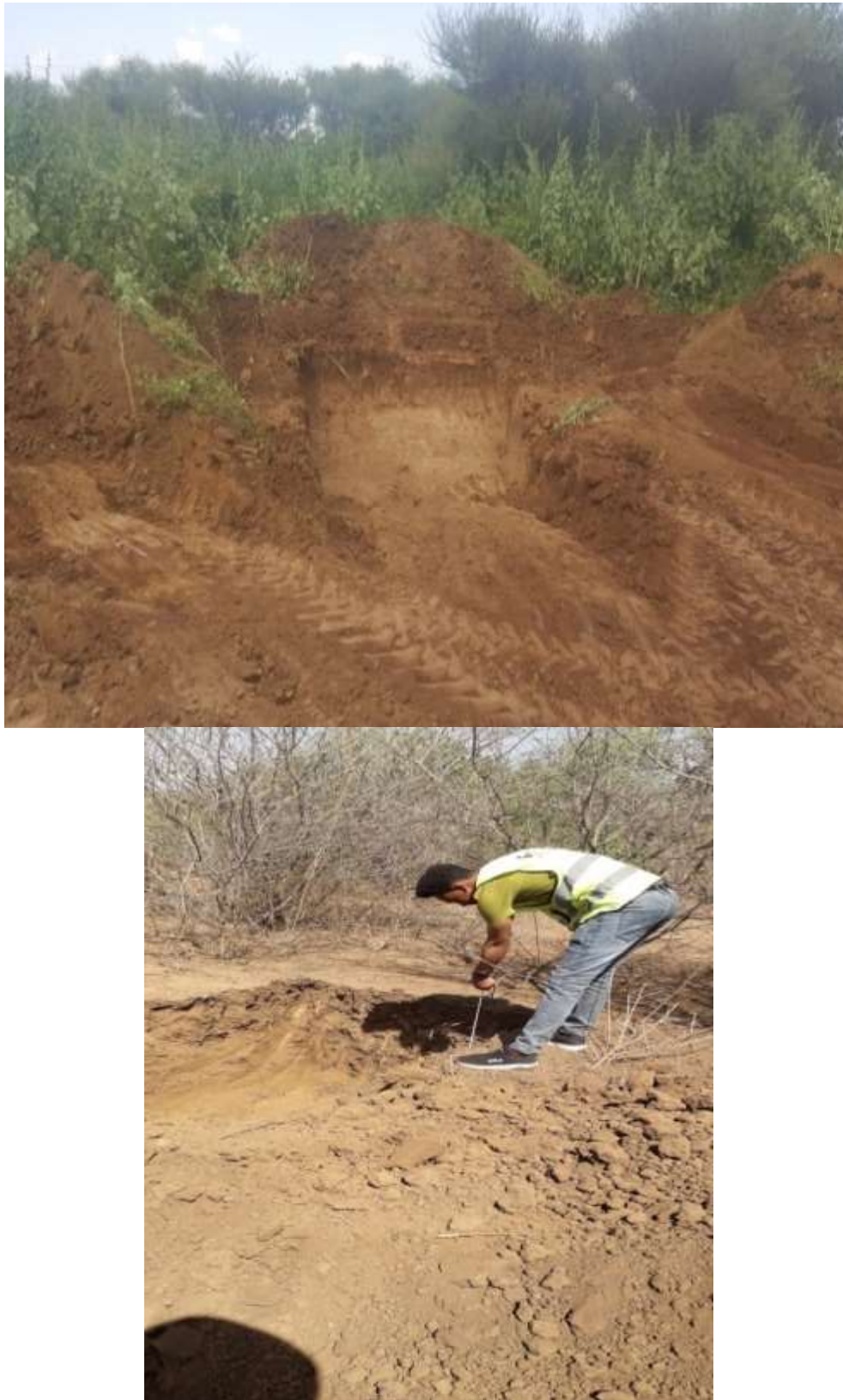
Figure 4-1 Typical test pits photograph
