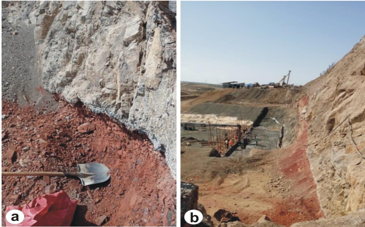
Plate 4.2 Soil sampling locations (a) Test pit (TP-1) at the core termination in between porphyritic basalt above and aphanitic basalt below on the right abutment of the dam and (b) The core termination at the right abutment in contact with paleo-soil and line of conduit outlet work structure.
