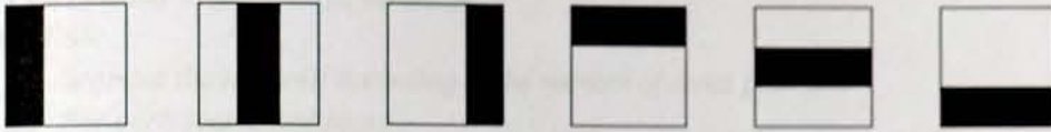
Figure 3.6: Different combinations of black pixels that result the same value for a zone
