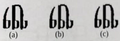
Figure 4.11: Interpolation methods applied to the character “aa.” (a) Nearest (b) Bilinear (c) Bi-cubic
