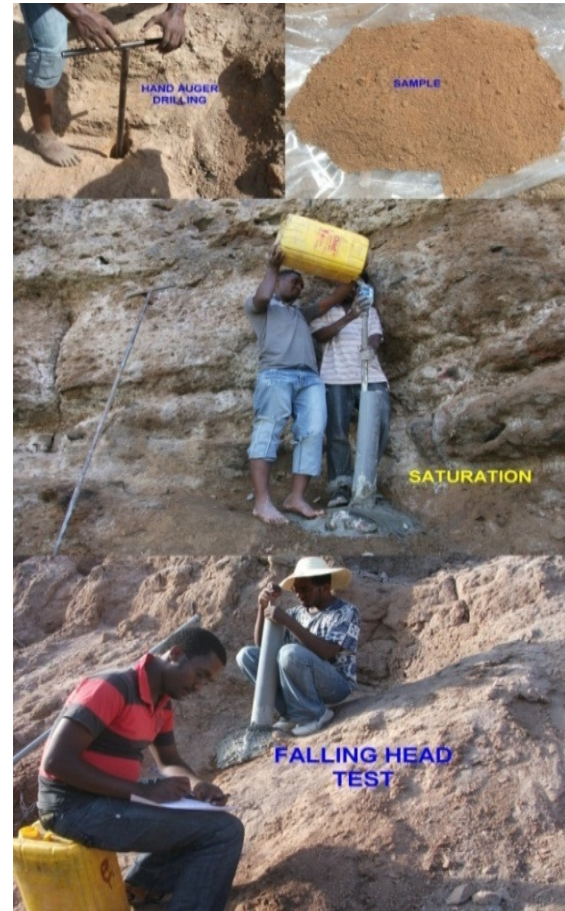
Plate 5.2 In situ falling head permeability test on tuff
