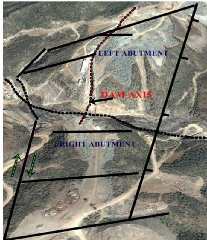
Plate 2.2. Major and minor faults in and around dam site and their interconnection for leakage path At the dam site, several faults were traced crossing the dam axis nearly perpendicular and having extension in to the reservoir. These faults are threats for stability and excessive water loss. To amend
