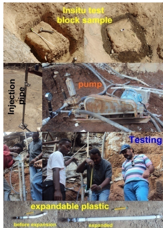
Plate 5.3 Insitu permeation test
