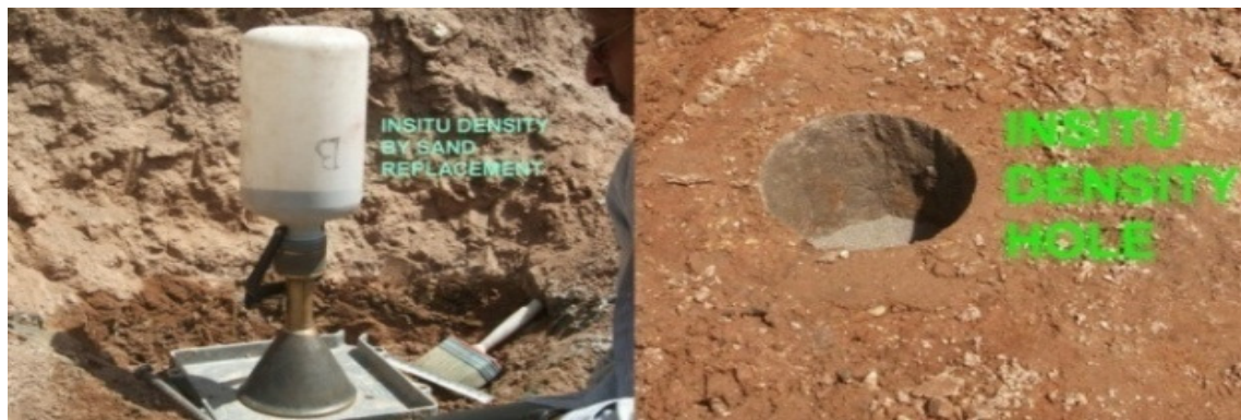
Plate 5.1 Insitu density test on tuff
