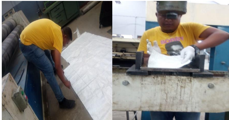
Figure 3. 6 prepare measuring and cutting of the glass fiber to prepare the sample
