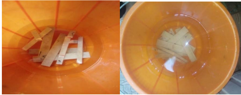
Figure 4. 10 Specimens Immersed in Distilled Water
