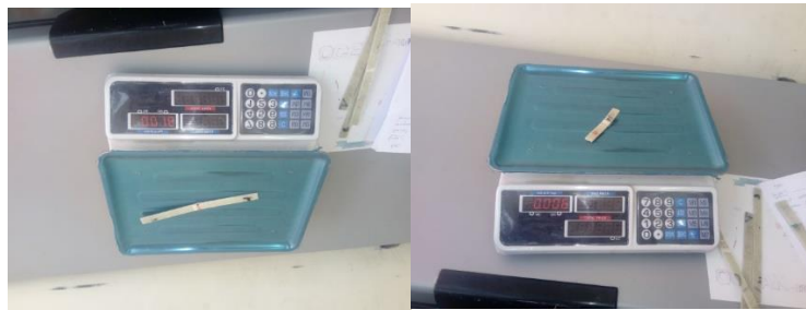
Figure 4. 9 measuring of specimen before and after water immersion
