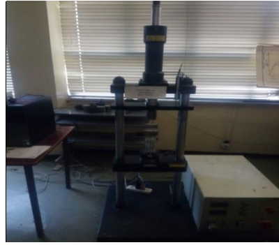
Figure 3. 11 Universal testing machine testing machine model WP 310
