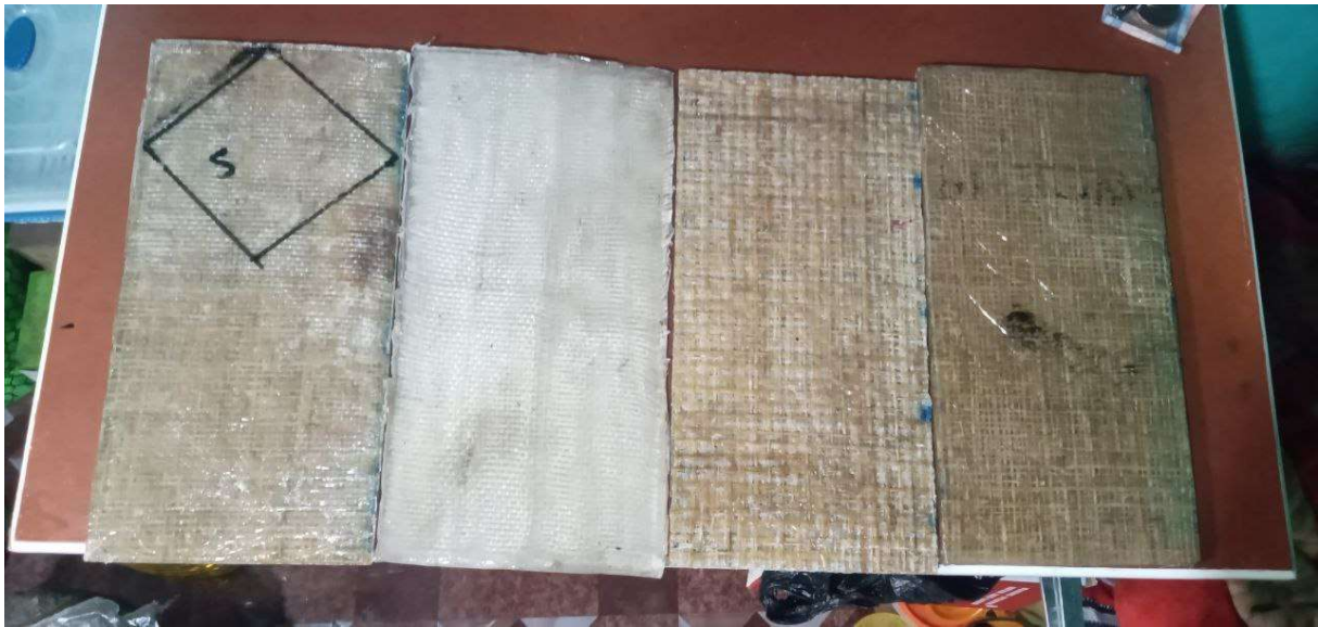
Figure 14: Fabricated composite laminates: interply hybrid, pure glass, intraply hybrid, and pure sisal composite laminate (from left to right)
