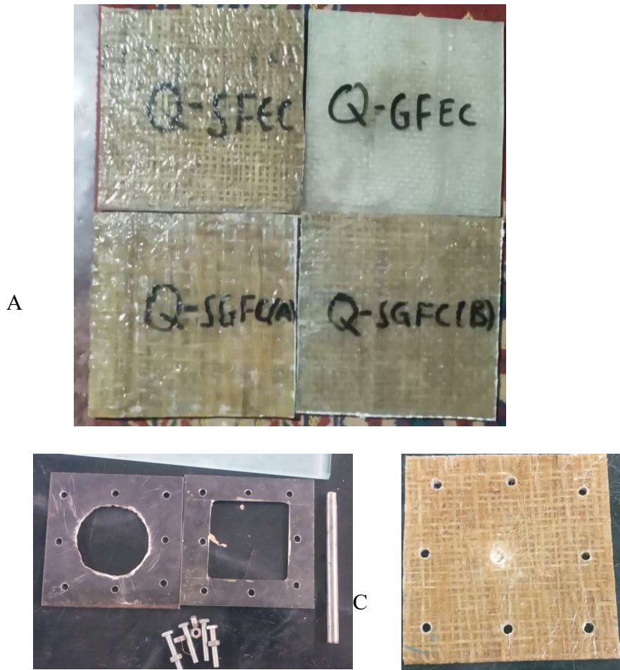
Figure 17: Quasi static penetration test (A) Cut specimen, (B) Fixture, and (C) Drilled specimen
