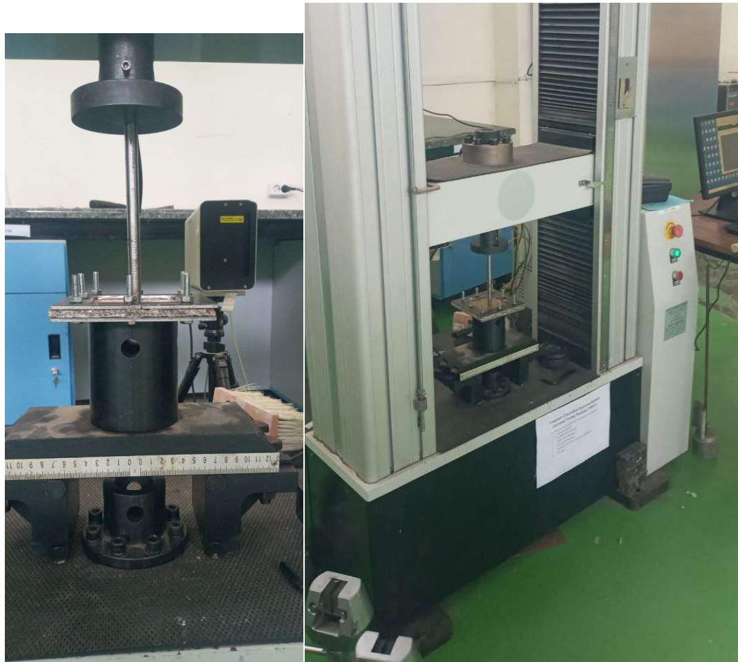
Figure 22: Quasi-static penetration test setup
