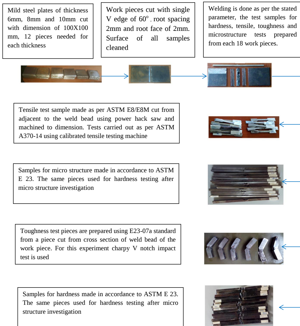
Figure 8: Process flow chart for test piece preparation
