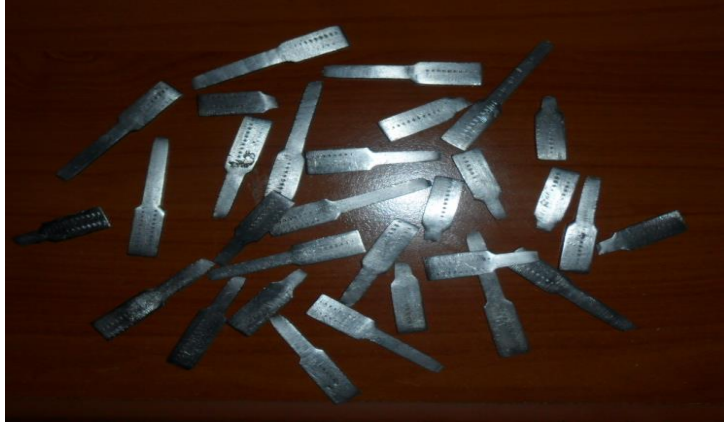
Figure 17: Tensile test pieces after destructive testing
