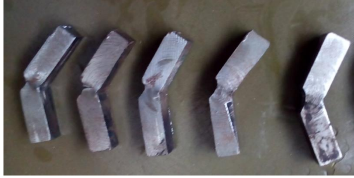
Figure 20: Toughness test pieces after impact test
