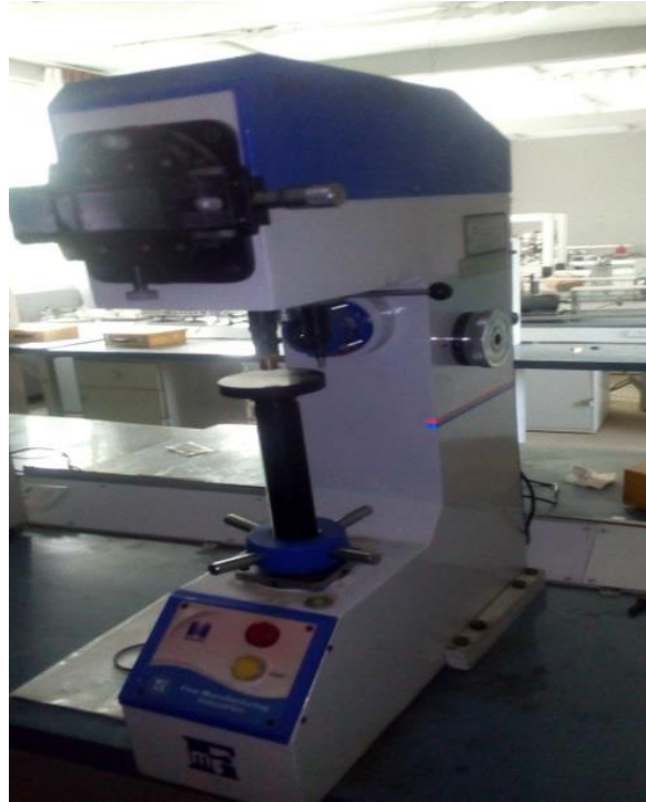
Figure 12: Vicker's hardness testing machine used for hardness test
