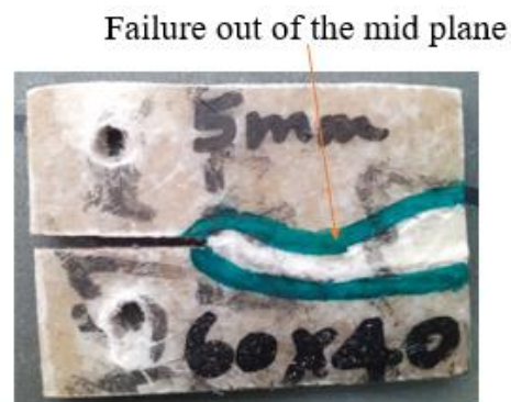
Figure 33: Failure modes in compact tension tested specimen
