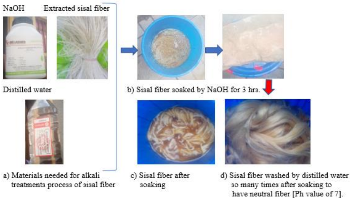
Figure 16: Alkali treatment of sisal fiber
