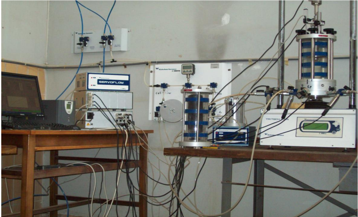
Figure C-1: A Picture of Triaxial Test Apparatus in AAU soil Laboratory
