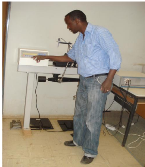
Figure C-2: A Picture of Direct shear apparatus in AAU soil Laboratory
