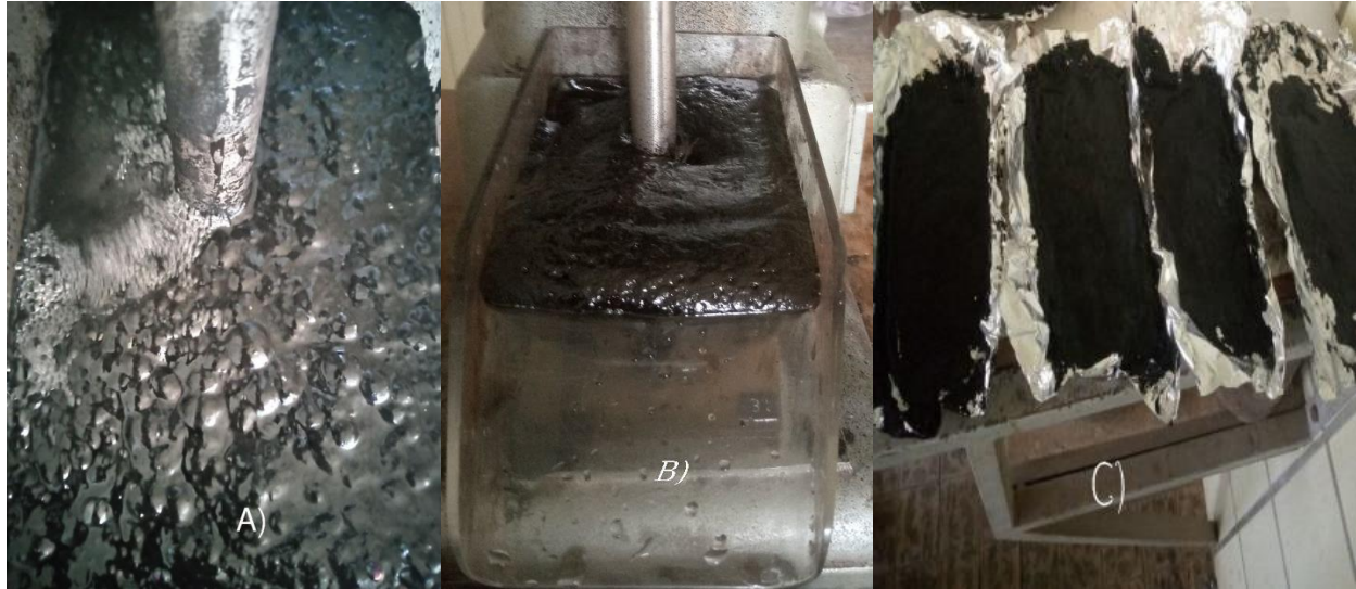
Figure 5: The procedures for froth flotation and the resulting coal particles.
