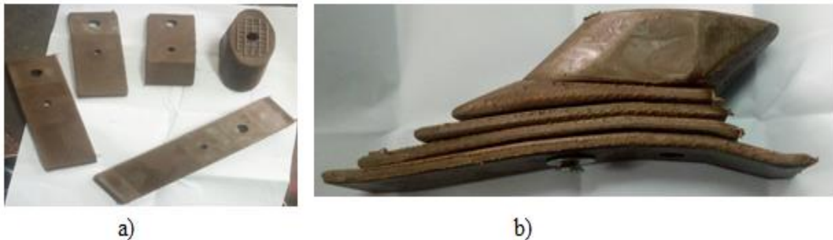
Figure 4. 16 a) blades and keel, b) Assembly of prosthetic foot (Source: POC Ethiopia)
