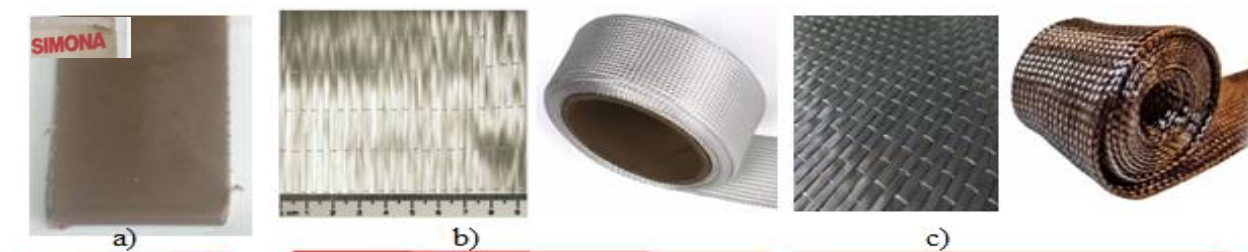
Figure 4. 20 Material used a) HPP b) E-glass and c) Carbon fiber [55]
