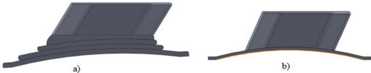
Figure 4. 18 A 3D assembly model of prosthetic foot in SOLIDWORK: a) HPP, b) Composite
