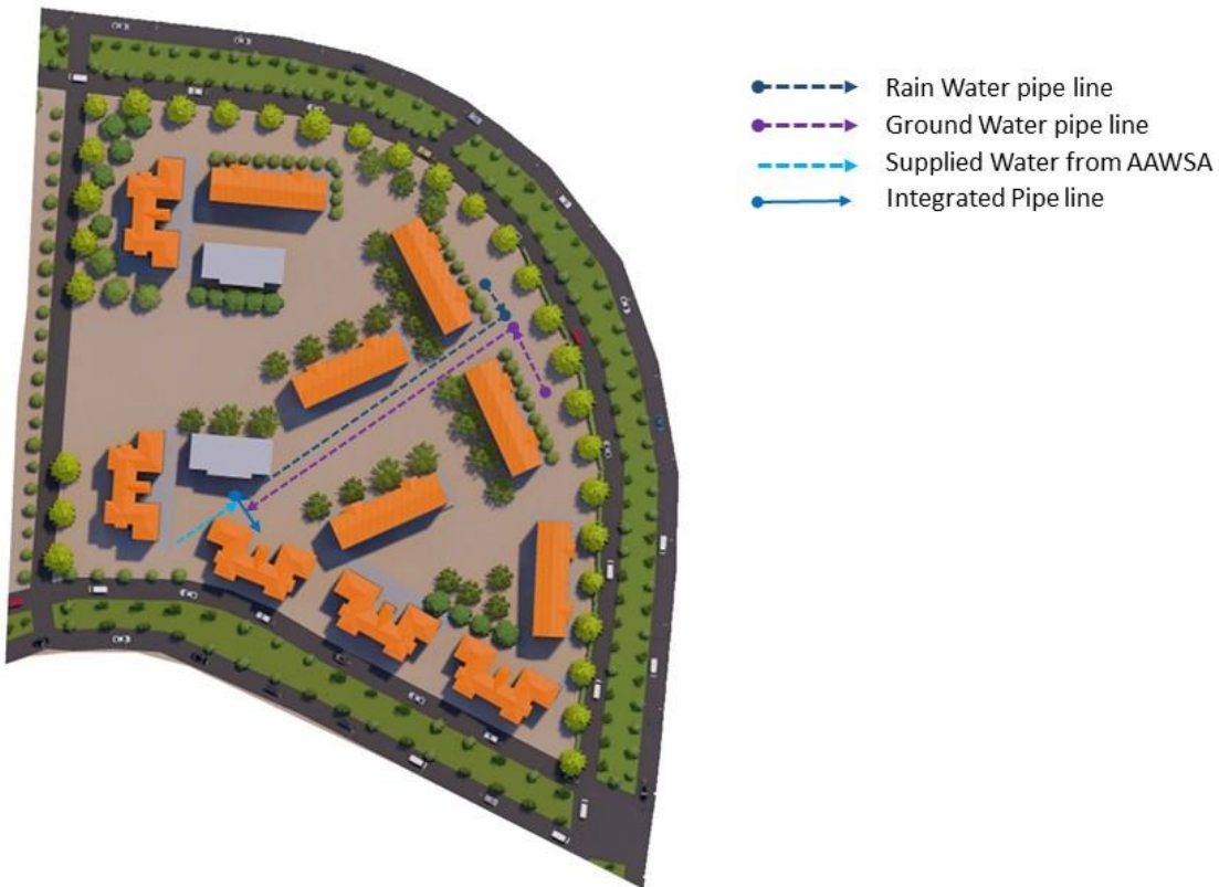
Figure 0.35: Piped Water Supply System Integration
