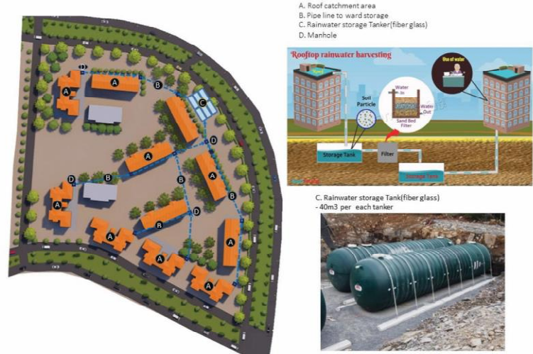
Figure 3. Collection and storage mechanism of rainwater
