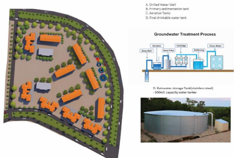
Figure 4. Extraction and treatment mechanism of groundwater
