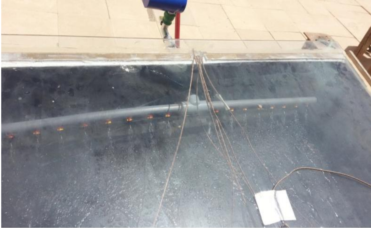
Figure 2. 16: Water film cooling of the glass cover [14]
