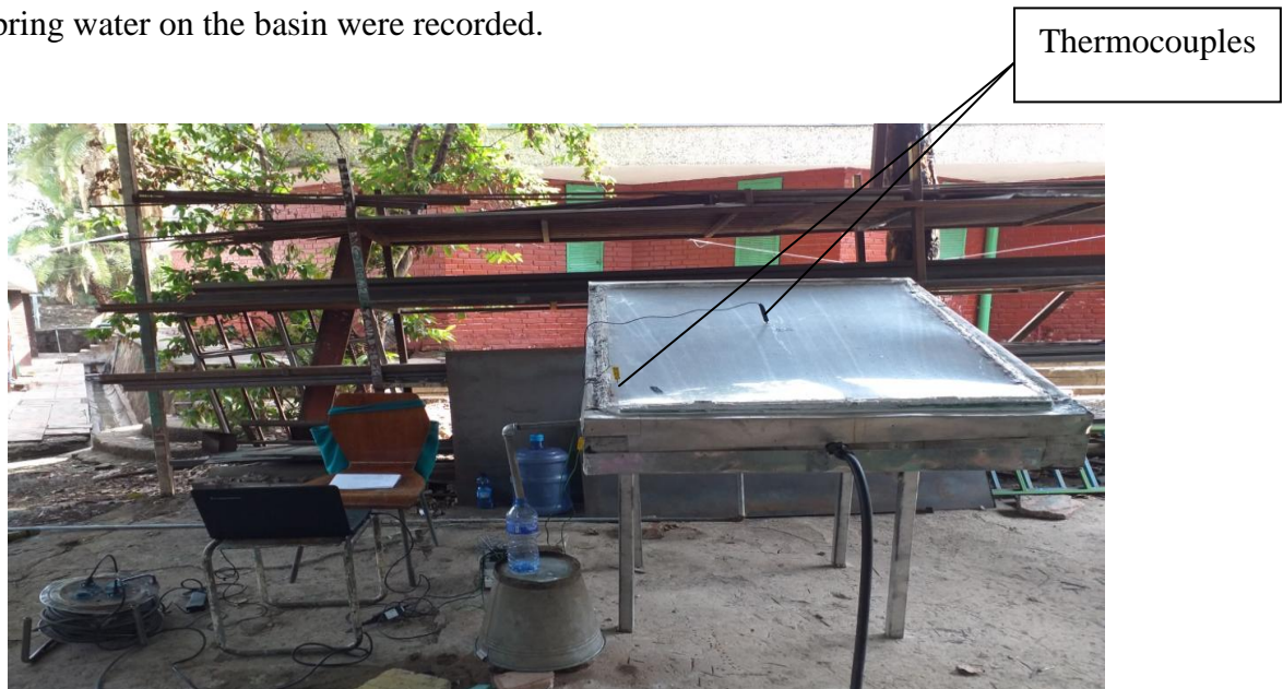
Figure 3. 21: Thermocouples inserted through the glass cover
