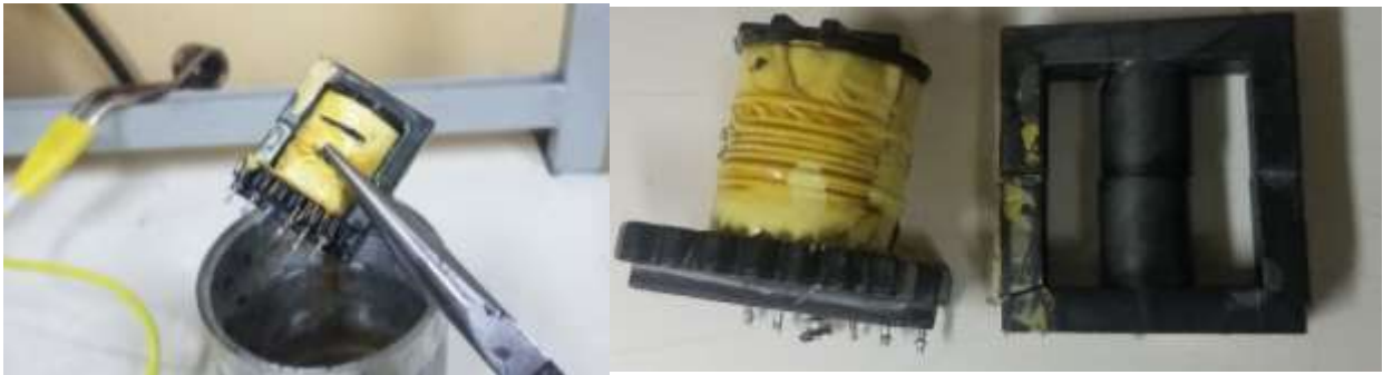
Figure 47 Ferrite transformer Dismantling
