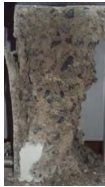
Figure 4.1 Failure of Unconfined Concrete Column
