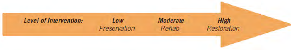
Figure.-14.Intervention for deterioration of historic buildings
