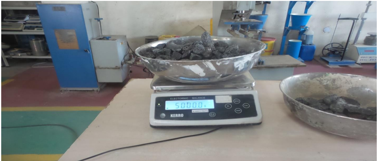
(b): Ballast weighting
