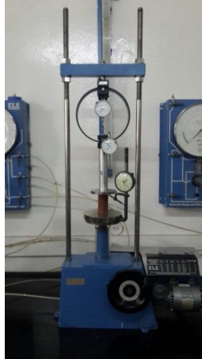
Figure 2.1 Unconfined Compression test machine
