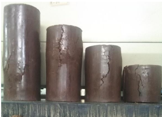
c) Sample remoulded at dry side of OMC
