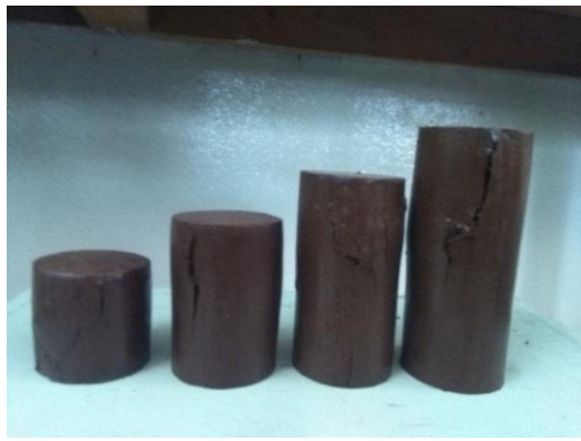
c) sample remoulded at dry side of OMC
