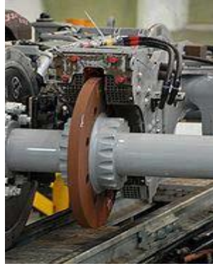
Fig. 3.14: Eddy-current disc brake on 700 Series Shinkansen (Johnson, 2012)
