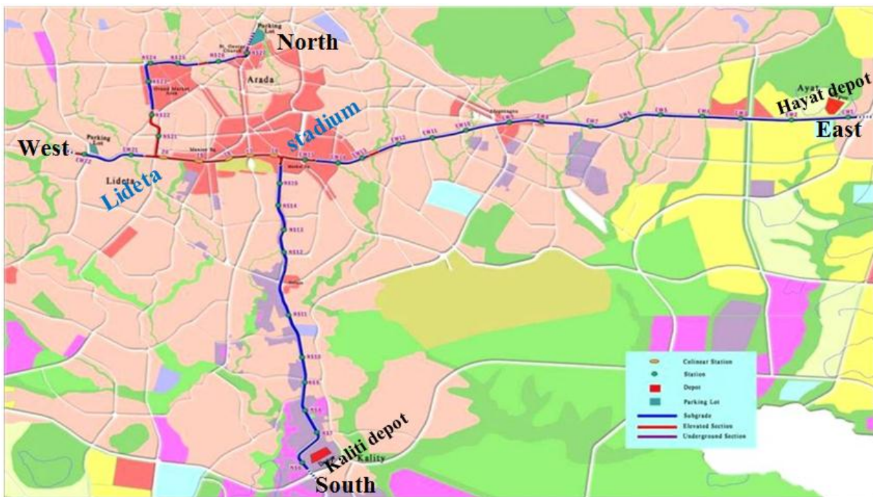
Figure 3.1: Addis LRT system topological drawing [7]
