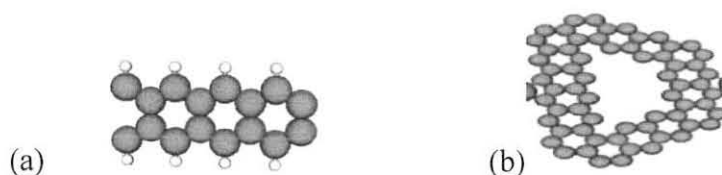
Figure 1.4.1 (a) A graphene nanostructure with symmetric edges and showing zero spin transport. (b) A graphene nanostructure with asymmetric edges and also a hollow dot (anti region) at the center, which is believed to show spin transport.
