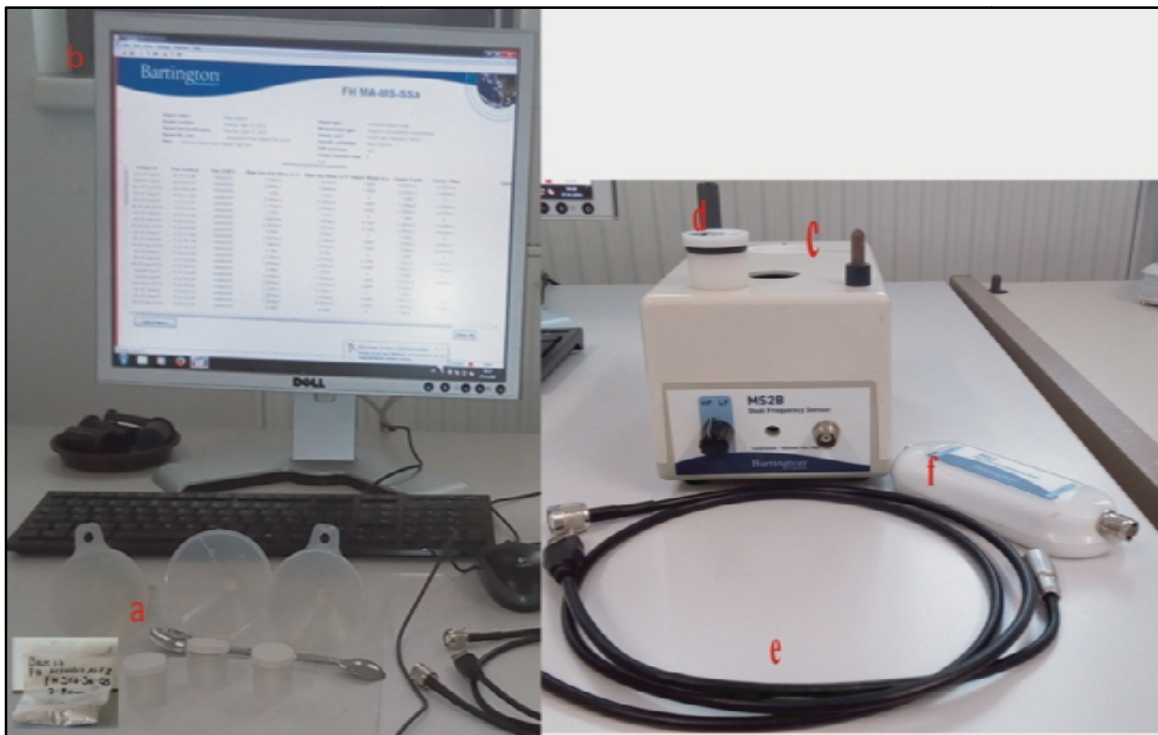
Figure 1.9. Equipment used to prepare and measure the magnetic susceptibility of sediment samples: (a) sediments sample and sample container; (b) computer with Bartsoft instrumentation Software; (c) MS2B sensor, d) cassette tape used to calibrate the sensor, (e) USB cables, and (f) MS3 meter.
