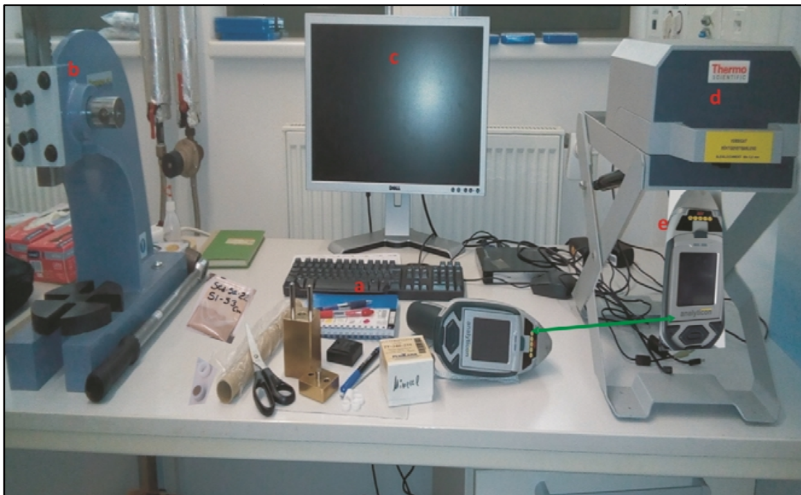
Figure 1.10. Equipment and analytical instruments used to measure the elemental composition of sediments: (a) different tools used to prepare the sediment samples including polypropylene thin films which helps to detect the lighter elements, notebook, plastic, pressed powder pellets, sample holder, and powdered sediment samples; (b) machine used to press the sediment samples and make it harder; (c) computer display with NITON and NDT program; (d) test stand used to hold the NITON XL3 Analyzer; (e) NITON XL3 Analyzer which is used to analyze the elemental composition of sediment samples.
