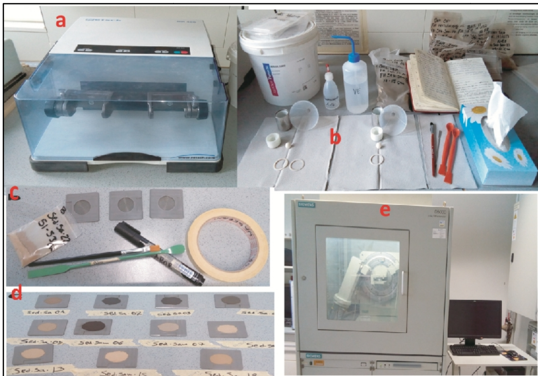
Figure 1.11. Equipment used to prepare and analyze the mineralogical composition of sediments: (a) Retsch Mini Mill (MM 400), used to mill the sediments; (b) sample holder, note book, sediment samples, and isopropanol, beach sand and de-mineralized water; all used to clean the equipments; (c) materials used to prepare sediment samples for the XRD analysis including sample holder pellets, plaster, powdered sediments sample, small shovel, brush, and marker pen; (d) prepared sample for XRD analysis; (e) X-ray diffractometer D5000 Analyzer and computer.
