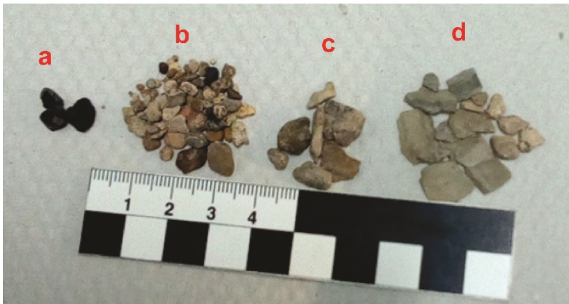
Figure 3.4. Rock fragments and ecofacts (charcoal) recovered from sieving on 2mm mesh size of sediments from lithofacies FHL-07 (FH SS 07 & FH SS 08). While, (a) charcoal, (b) different source (mixed) of rounded and poorly sorted grains, (c) black color, angular shaped fine grained rock fragments (i.e. aphanatic basaltic), (d) light color, fine-grained, angular shape rock fragments (trachytic).
