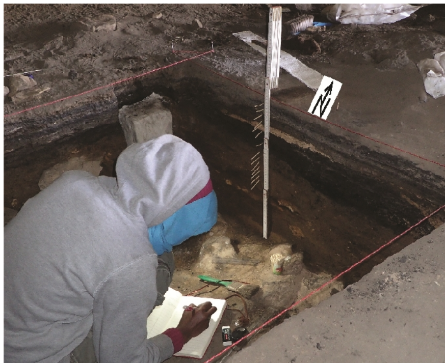
Figure 1.4. Field photograph of sediment samples collection and description from Fincha Habera section (Northern profile). Tooth picks are used as scale (i.e., to take a sample based on two centimeters), and materials used to collect the sediments include brush, shovel, plaster, plastic
