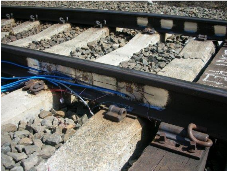
Figure 2-10: Railway track mounted with strain gauges[43]
