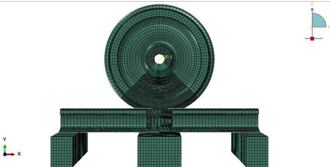
Figure 3-30: Assembled and meshed ABAQUS FE model of a coupled quarter car train-track system with a fined mesh at contact points.
