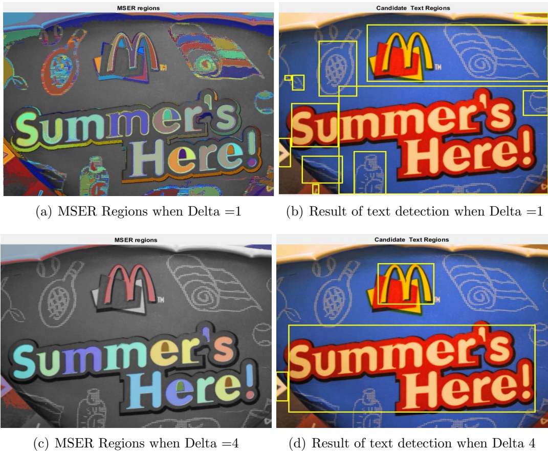
Figure 5.3: The effect of delta on the result of text detection through MSER.
