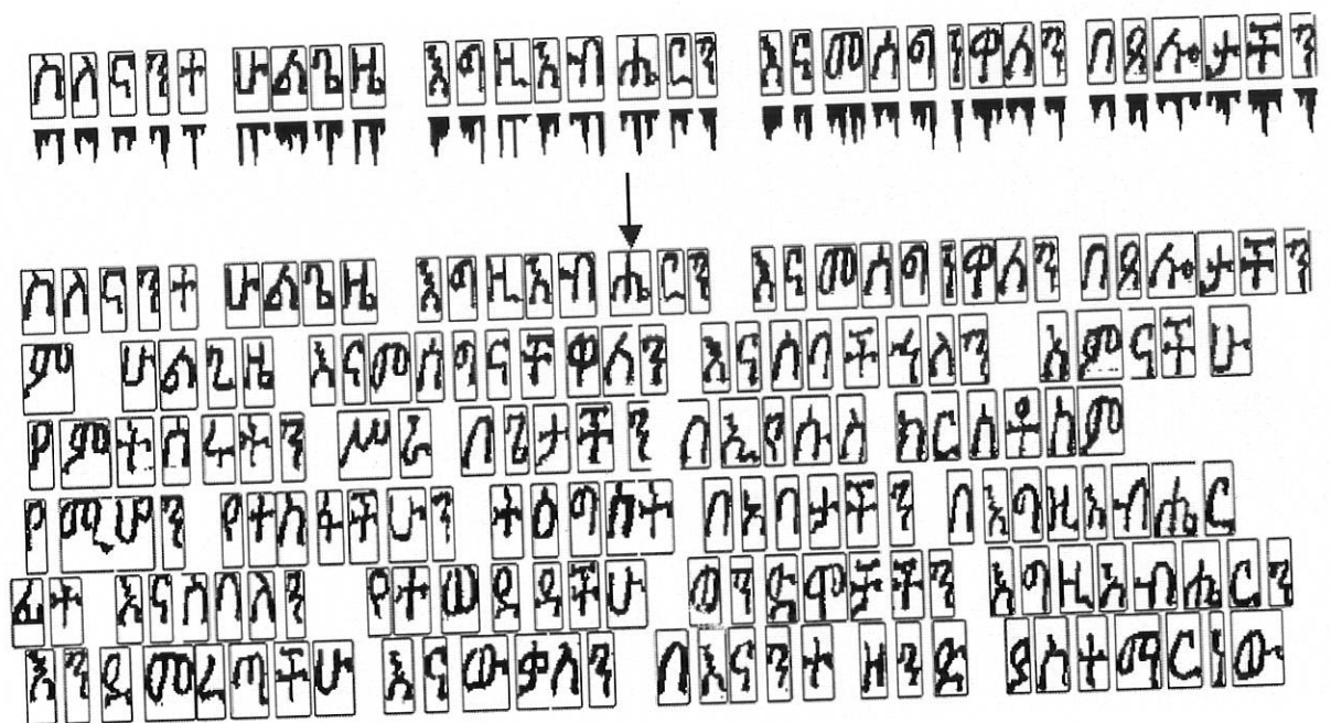
Figure 13: Sample Output of the Character Segmentation with Veridical Projection Profile
