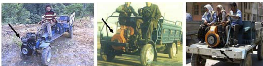
Figure 1.3 Three examples of auxiliary agricultural vehicle driven by the single cylinder diesel engine [9]
