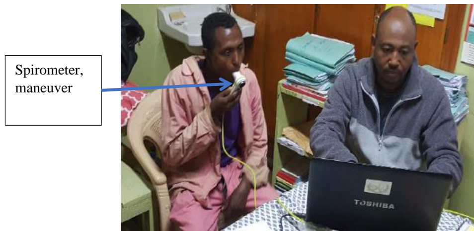
Figure 8: Cross-shift lung function test using a computer connected spirometer ( Source: Photo by Author)
