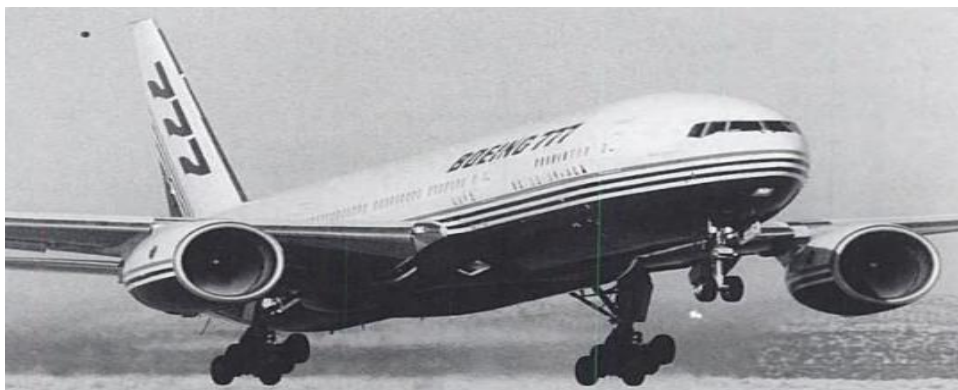
Fig 3.2 Boeing 777, the first American Commercial aircraft with composite empennage
